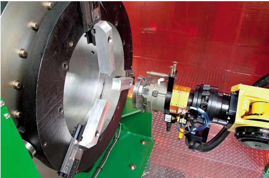
The end-ring is located in the second set of clamping jaws.
