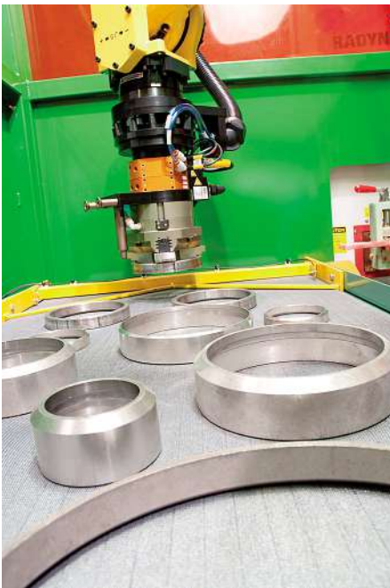
The robot picks up an end-ring from the feed conveyor belt.
