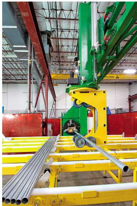
Via a hall portal crane, the tube, cut to the specified length, is picked up and introduced into the servo-controlled clamping device.
