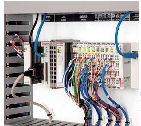
The Beckhoff CX1010 Embedded PC with Twincat NC PTP software controls the complete ARC 11 RB welding process.
