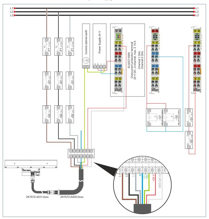
The following table shows the assignment for the XPlanar power cable:
