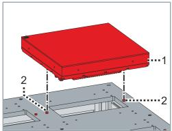
► Position the tile [1] with the locating pin hole and the elongated hole on the locating pins [2]
