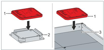
▶ Place the mover [1] in the transport securing device [2] with the upper side facing upwards
