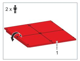
► Turn the frame [1] with attached assembly aids by 180°
