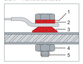
► Ground the painted surface with spring washer [1], washer [2], contact washer [3], nut [4] and bolt [5]
