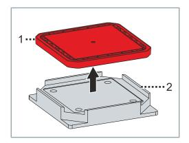
► Remove the mover [1] from the transport securing device [2] and rotate it by 180°
