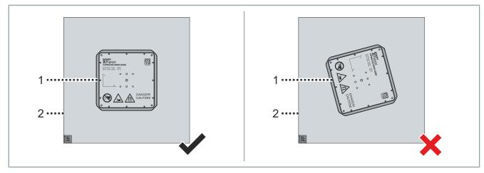
When placing the movers [1], ensure that they are positioned as parallel as possible to the outer edges of the tile [2].
