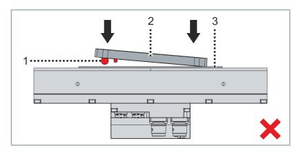
There must be no dirt or foreign objects [1] between the mover [2] and the cover [3] or the tile [4]. All dirt and foreign objects on the underside of the mover and on the surface of the cover or tile must be removed before force is applied to the mover.
