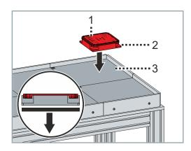
► Position the mover [1] with transport securing device [2] directly on the tile [3]
