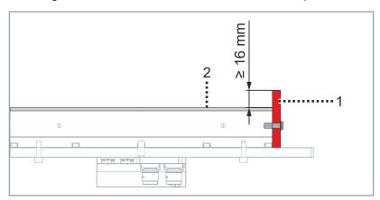
The mechanical protection [1] must protrude at least 16 mm beyond the stator surface [2].
