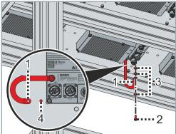
► Screw the cable lug of the ground strap [1] to the machine bed [4] using a screw [2] and washers [3]
