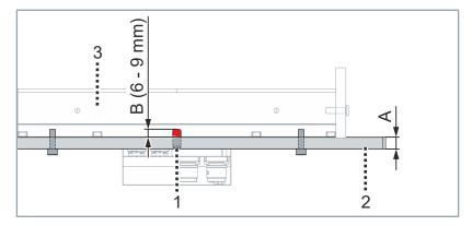
The length [C] of the D8 locating pins [1] for aligning the tile depends on the height [A] of the machine bed [3] and the projection [B] into the tile [3].
