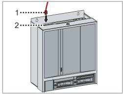
► Connect the connector of the EtherCAT G cable ZK1B96-819A-0xxx or ZK1B96-8191-0xxx to the industrial PC
