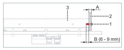
The length [C] of the M6 screws [1] for fastening the mechanical protection depends on the depth [A] of the safety equipment [2] and the screw depth [B] in the tile [3].
