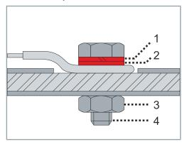
Ground the unpainted surface with spring washer [1], washer [2], nut [3] and bolt [4]
