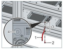
Screw the cable lug of the ground strap [1] to the functional earth connection [4] of the tile using a screw [2] and washers [3]
