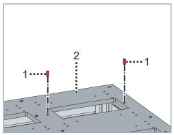
▶ Insert all locating pins [1] into the machine bed [2]
