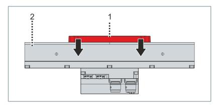
If the movers [1] are actively attracted to the tile [2] by a position specification of  $\leq 0$  mm, temperature peaks can occur. Monitor the temperature of the tile in the corresponding applications.
