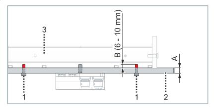
The length [C] of the M6 screws [1] for fastening the tile depends on the height [A] of the machine bed [2] and the screw depth [B] in the tile [3].
