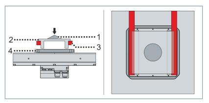
If a product [1] is to be applied with force to a workpiece carrier [2], the workpiece carrier must rest on an anvil [3]. While the workpiece carrier is resting on the anvil, the mover [4] can be lowered.
