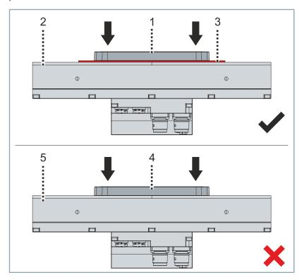
If you want to perform press-in processes on the mover, you must fit a cover [3] between the mover [1] and the tile [2].
