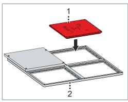
► Insert the mover [1] into the frame [2]
