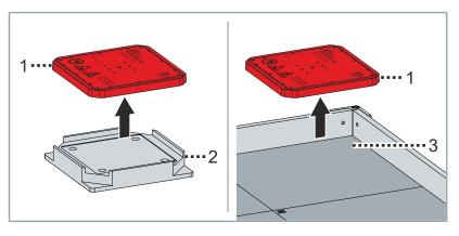
► Remove the mover [1] from the transport securing device [2] and rotate it by 180°
