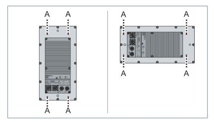
Locating pins for installing the tiles
