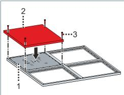
➤ Secure the mover [1] with the assembly aid [2] and four screws [3] to prevent it from falling out
