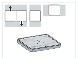
Once placed on the tiles, the movers move highly dynamically on the top surface of the tiles. Collisions are avoided. Movers can be raised, lowered and tilted while in motion. The movers are available in the following versions:
