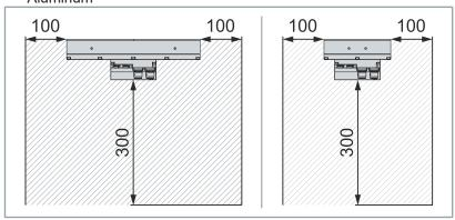
No magnetic materials may be used within a distance of 100 mm around a tile and 300 mm below a tile.
