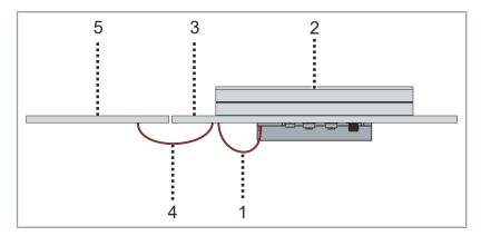
The functional conductor connection [1] of the tile [2] must be connected to the machine bed [3]. In addition, the machine bed [3] must be connected to another machine bed [5] with a functional conductor connection [4].
