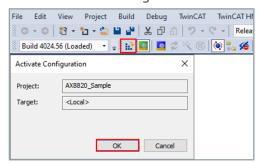
The selected settings take effect when the configuration is activated. The parameter settings are also saved in the EEPROM of the AX8820 by activating the configuration. The AX8820 is fully functional if the EtherCAT connection is interrupted.
