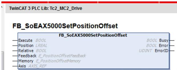
A PLC function block is available in the library **TC2\_MC2\_Drive** under TwinCAT 3 for saving or modifying the offset from a user program:
