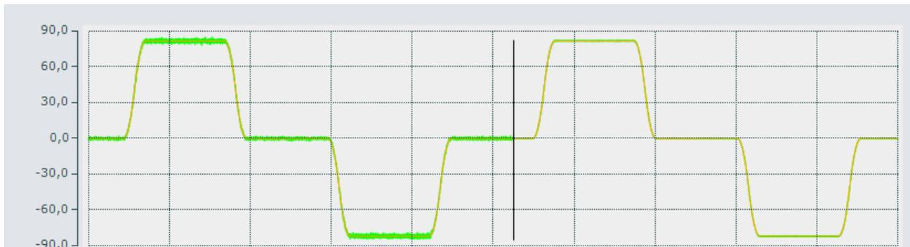
The recording originates from a linear axis with ball screw. The green line shows the actual velocity in mm/s. The Observer was activated at the black vertical line.
