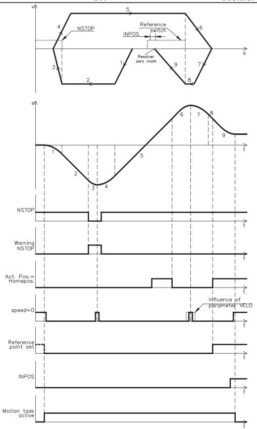
After the homing run has been completed, Bit 11 STW must be set to 0 again.
