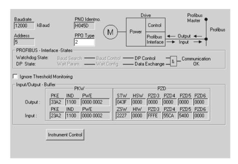
**Baudrate:** The baud rate set by the PROFIBUS master.
