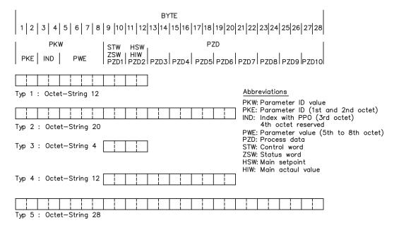
AX2000/2500 only uses the PPO-type 2 (with 4 words PKW-section and 6 words PZD-section). The PKW-section is used mainly for the transmission of parameters for the servo amplifier, the PZD-section is used principally for handling motion functions.
