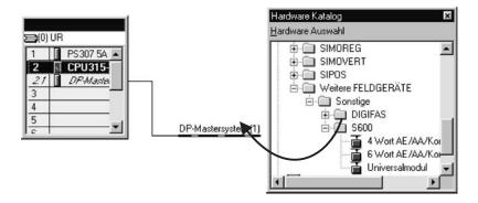
Next, use the same method as above to drag the module from the Hardware catalog into the box for the field unit, whereby the 4-word module must lie in Cell 0 and the 6-word module in Cell 1.
