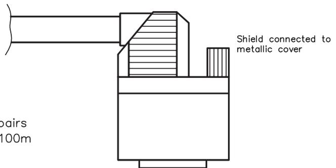
Shield connected to metallic cover
