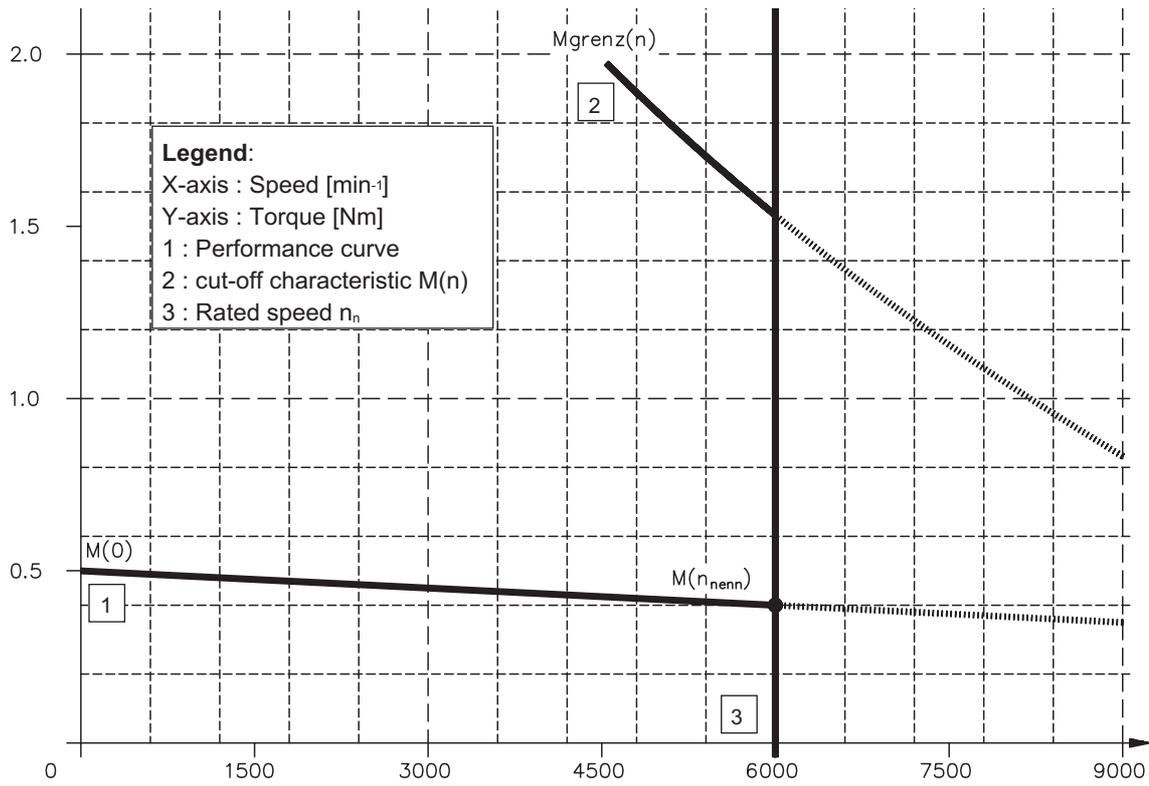
III.9 Torque characteristics AM237M
