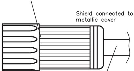
Shield connected to metallic cover
