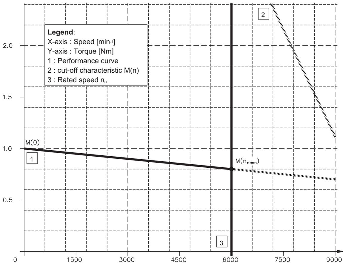
III.10 Torque characteristics AM237L
