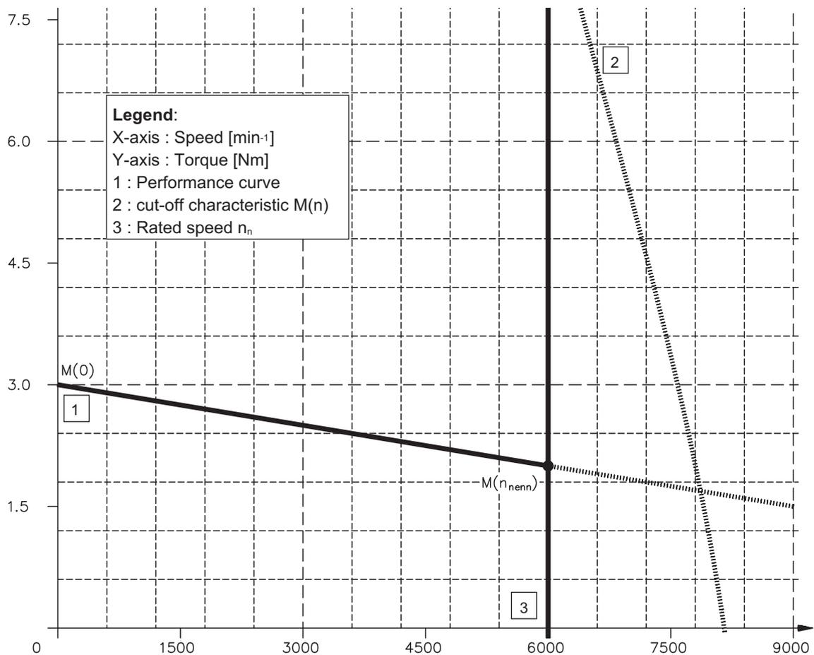
III.12 Torque characteristics AM247L
