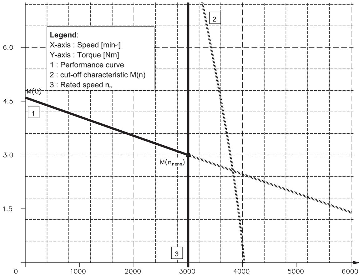
III.14 Torque characteristics AM257M
