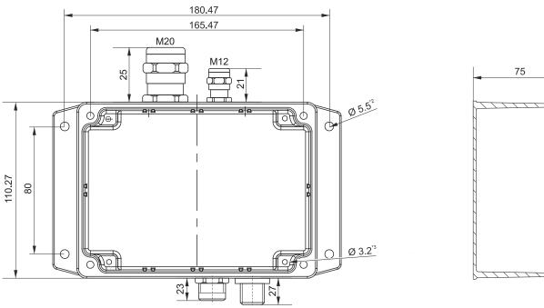
2\*) The holes on the mounting lugs are provided for M5 flat head screws.
