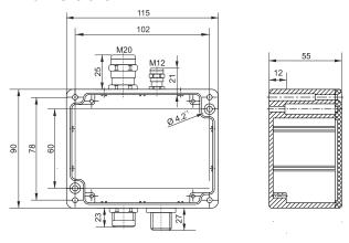
$1^*$ ) The holes with the diameter Ø 4.2 are provided for mounting the connector box. The holes are provided for M4 flat head screws DIN 7984.
