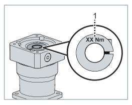
The value for the tightening torque [1] of the clamping screw is punched into the clamping hub from above.
