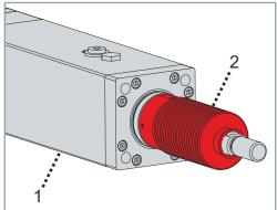
► Slide the bellows and flange fastening [2] onto the flange of the electric cylinder [1]
