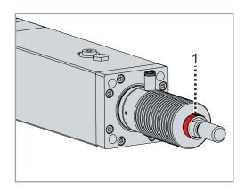
► Place the hose clamp [1] over the front end of the bellows and tighten with suitable pliers
