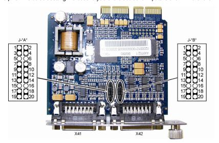
The opposite figure shows the basic jumper configuration, which is the same for channel A and channel B. The pins of input sockets X41 and X42 are wired firmly to the corresponding pins of the jumpers rows. The non-configurable pins are not shown. To use the additional inputs proceed as follows:
