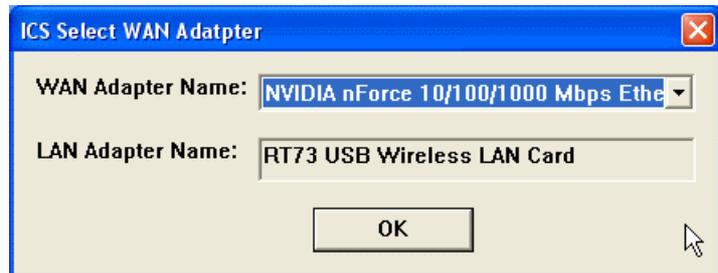
Select the WAN adapter and click *OK*. The *Ralink Wireless Utility* window appears and you can type the network name (*SSID*) and the channel.
