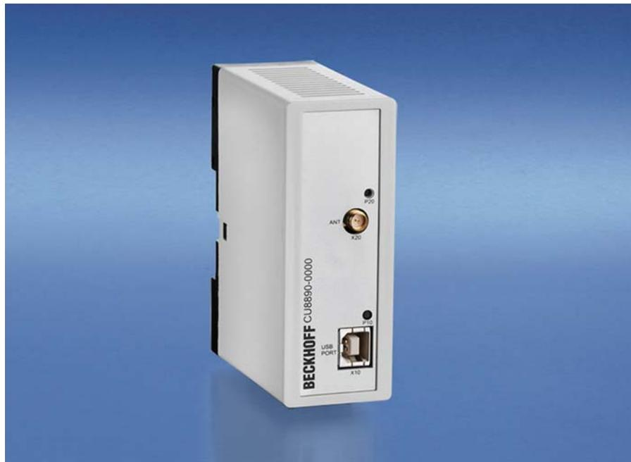
The CU8890 WLAN controller is an industrial grade data exchange unit for radio technology. The CU8890 is based on the standard IEEE 802.11 b/g and is designed for control cabinet installation. Connected to a Beckhoff Industrial PC the CU8890 can be used either as access-point or as client. Client drivers are available for Windows XP, XP Embedded as well as Windows CE, thus for each Beckhoff IPC as well as the CX-series. These support also adhoc modus.
