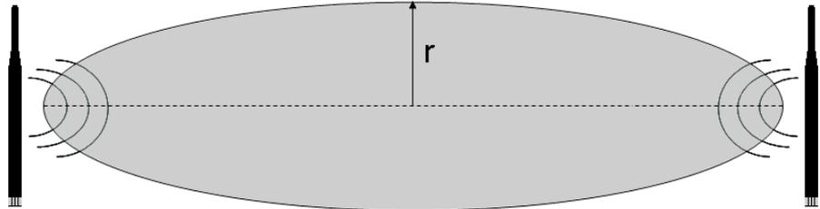
The main portion of the energy is transmitted in the area of the Fresnel zone.
