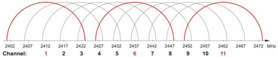
When using the network in a confined area (e.g. in a factory building) notice the following comb-shaped structure with a channel difference of 5 channels to each neighbor cell:
