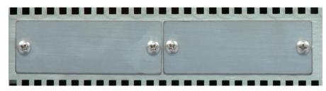
For the installation of the plug in cards first remove the cross-head screws. The cover caps can now be removed and allow plugging in the plug in cards.
