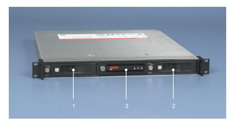
The C5210 is fitted with two removable frames for hard disks (1) and (2). In condition of delivery one of the removable frames is fitted with a hard disk. Behind the flap (3) the control elements and two USB-interfaces are located.
