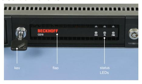
The control elements are located behind a flap at the front side of the Industrial PC. After unlocking the flap with the key it can be folded down. You now have access to the control elements:
