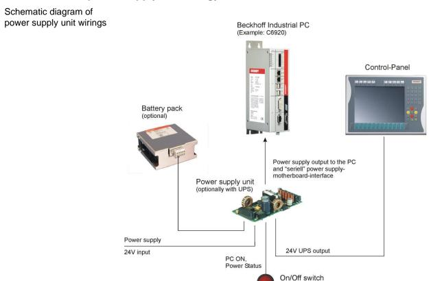
Industrial PCs equipped with a UPS are in actual use frequently switched off by simply turning off the supply voltage. In this case the PC shuts down via the battery. However, over time this reduces the service life of the battery.
