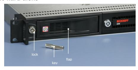
The hard disks are located into two removable hard drive racks at the front of the Industrial PC. After unlocking the flaps of the removable racks you can swivel out the hard disks. Now the disks can be removed.
