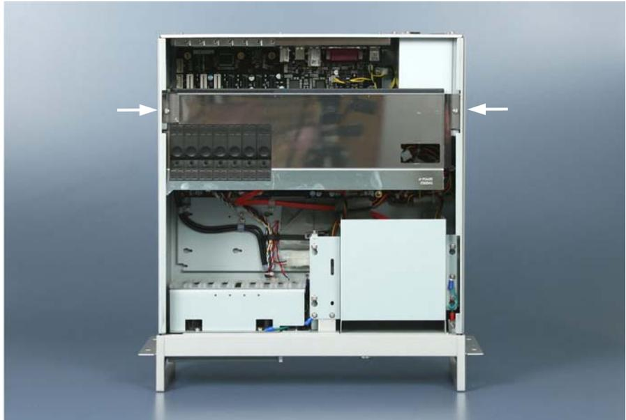
Remove the 2 fastening screws of the card holder (see arrows) using a cross-head screwdriver. The holder can then be lifted up.
