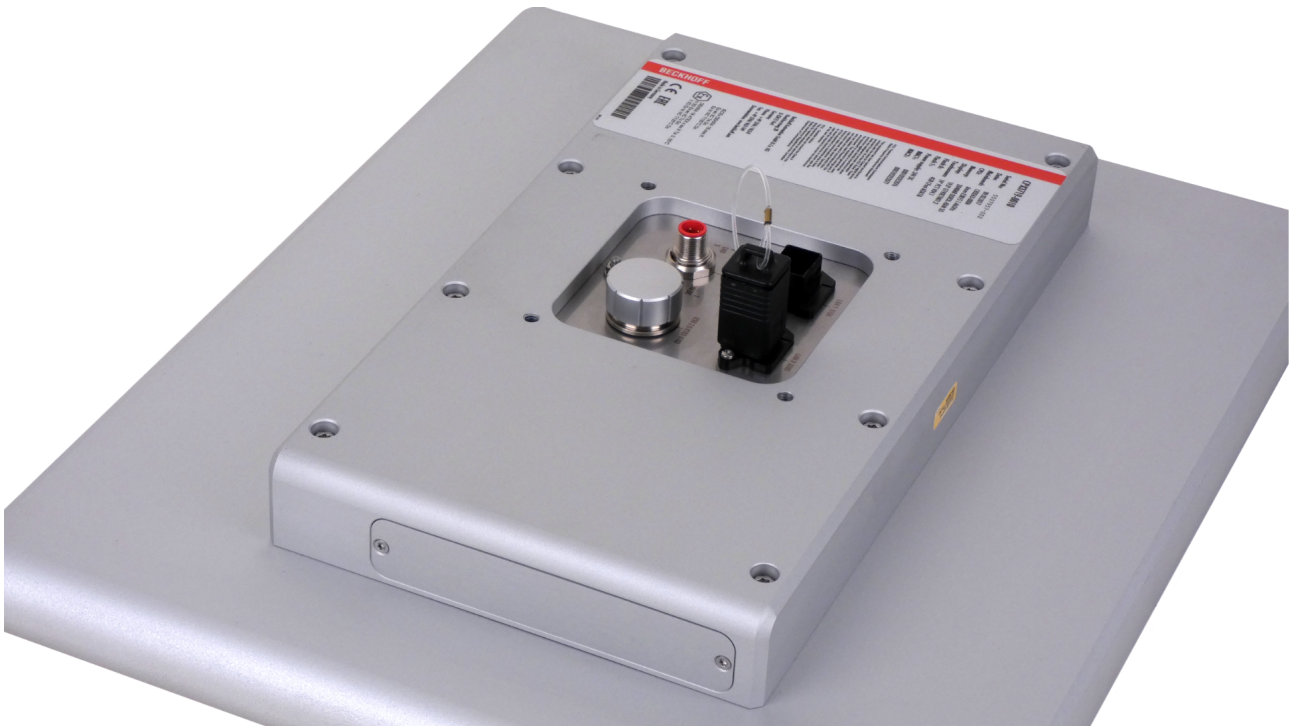
Fig. 2: CFAST card slot and battery of the system clock behind the cover plate
