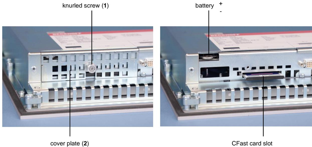
For replacing the battery and installation of the CFast card first unloose the knurled screw (1). The cover plate (2) can now be removed.
