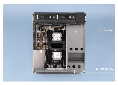
After loosening the knurled screw the card holder can be lifted off.
