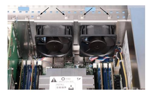
After removing the phillips head screws the fans can be exchanged. Therefor disconnect the supply cable from the motherboard.
