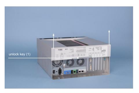
The housing cover is locked by a latch. After pressing the key (1) the cover can be fold up a little in the region of the connectors.
