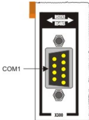
The CX50x0-N030 system interface provides an RS232 interface, COM1 (X300). It is implemented on a 9-pole Sub-D pin strip. If more than one interface is required the system can be extended via the Terminal Bus (K- or E-bus) or Bus Terminals (KL/EL6001) which provide serial interfaces. The pin assignment is shown at the bottom of the page.
