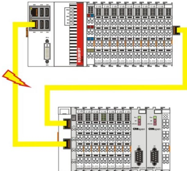
In this case the second cable is faulty. The terminals at the coupler continue to run without malfunction. The System Manager indicates the behavior as follows:
