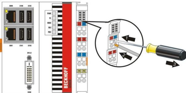
The terminals are implemented in spring force technology. Connect the cables as follows:
