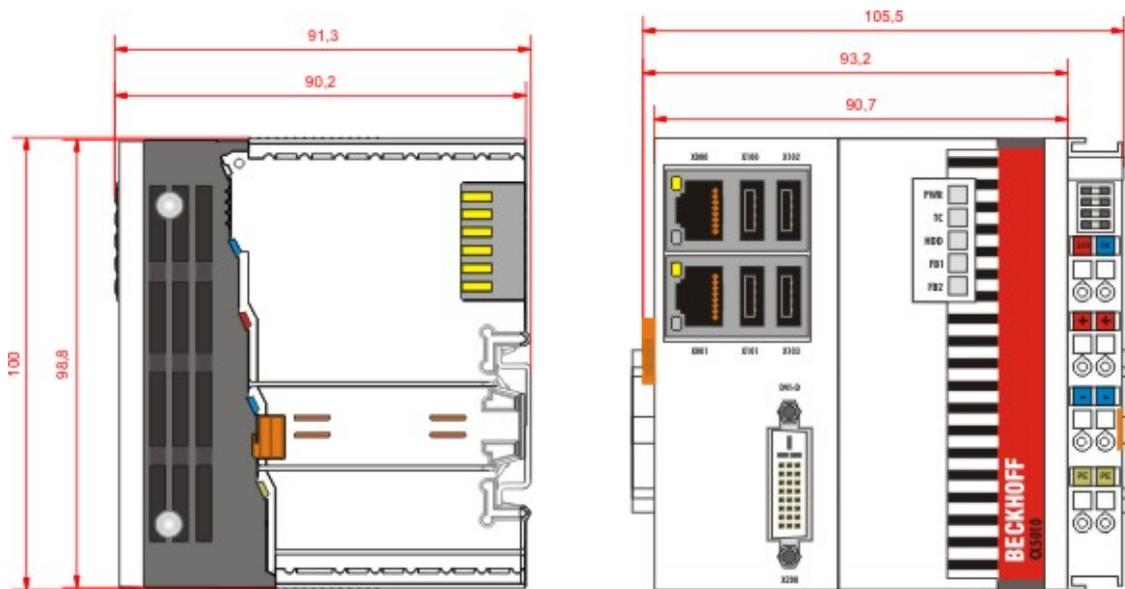
The basic configuration of the CX5010 includes a 128 MB Compact Flash card. The basic configuration includes two Ethernet RJ-45 interfaces, four USB-2.0 interfaces and a DVI-D interface.
