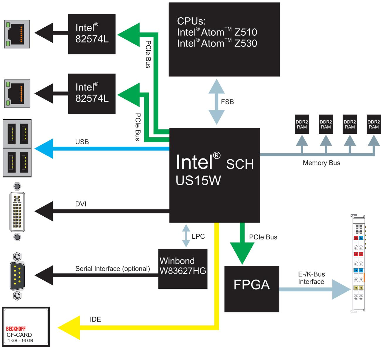
The CX50x0 Embedded PCs are based on the Intel Atom microarchitecture, which was developed by Intel. The CPUs used in the CX50x0 family are:
