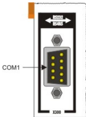
The CX50x0-N031 system interface provides an RS422 or RS 485 interface, COM1 (X300). It is implemented on a 9-pole Sub-D socket strip. If more than one interface is required the system can be extended via the Terminal Bus (K- or E-bus) or Bus Terminals (KL/EL6021) which provide serial interfaces. The pin assignment is shown at the bottom of the page.
