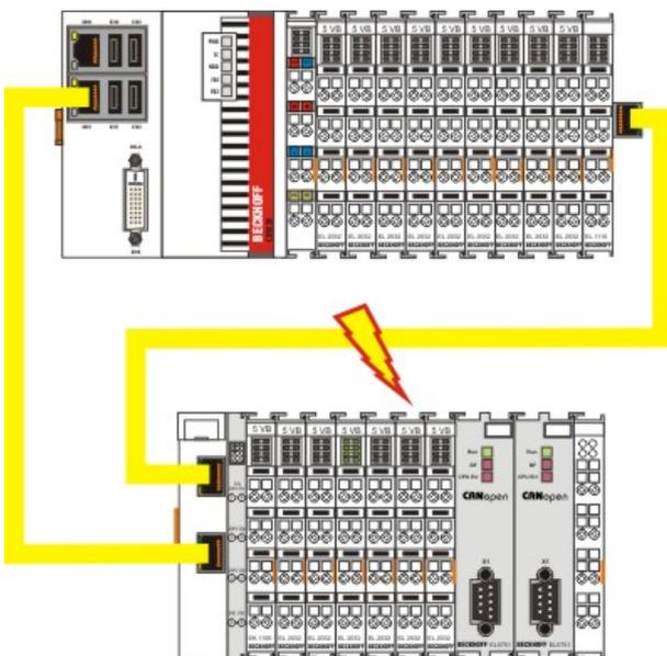
In this example the supply line for coupler EK1100 is faulty. The EK1100 terminals continue to run despite the cable failure. The System Manager indicates the failure as follows:
