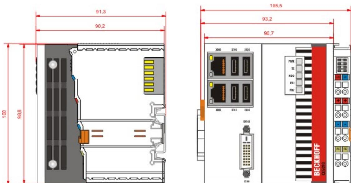
The basic configuration of the CX5020 includes a 128 MB Compact Flash card. The basic configuration includes two Ethernet RJ-45 interfaces, four USB-2.0 interfaces and a DVI-D interface.
