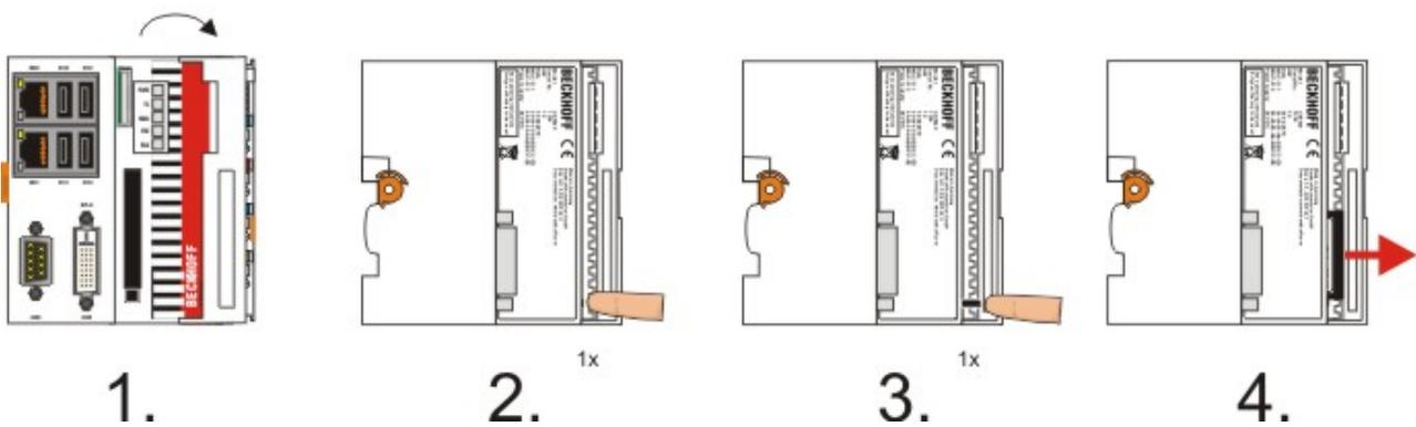
When the card is pushed back the eject mechanism locks again. The card is positioned correctly, if it is located approx. 1 mm lower than the front of the housing.
