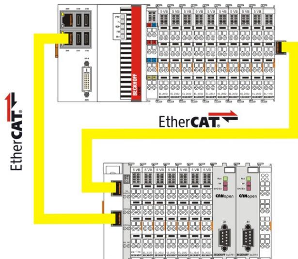
EtherCAT cable redundancy can be realised in the CX50x0 systems through the two independent Ethernet ports. Minimum requirements:
