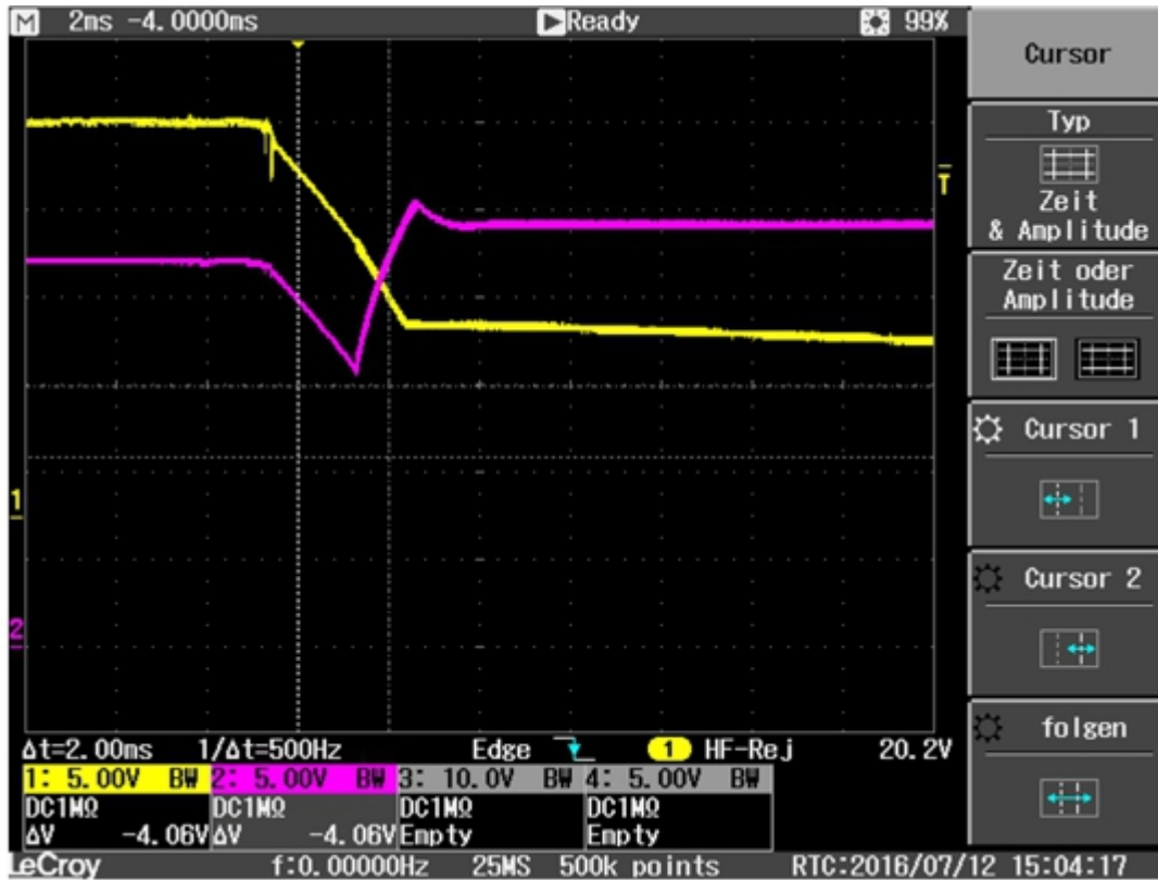
Fig. 3: Behavior in case of a power failure, oscillogram of the CX2100-0914 power supply unit.
