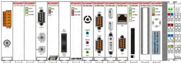
The light bus is shorted by a fiber optic cable. The PROFI bus master connection is connected to a BK3100 with terminals. The retention times are measured in relation to switch setting.
