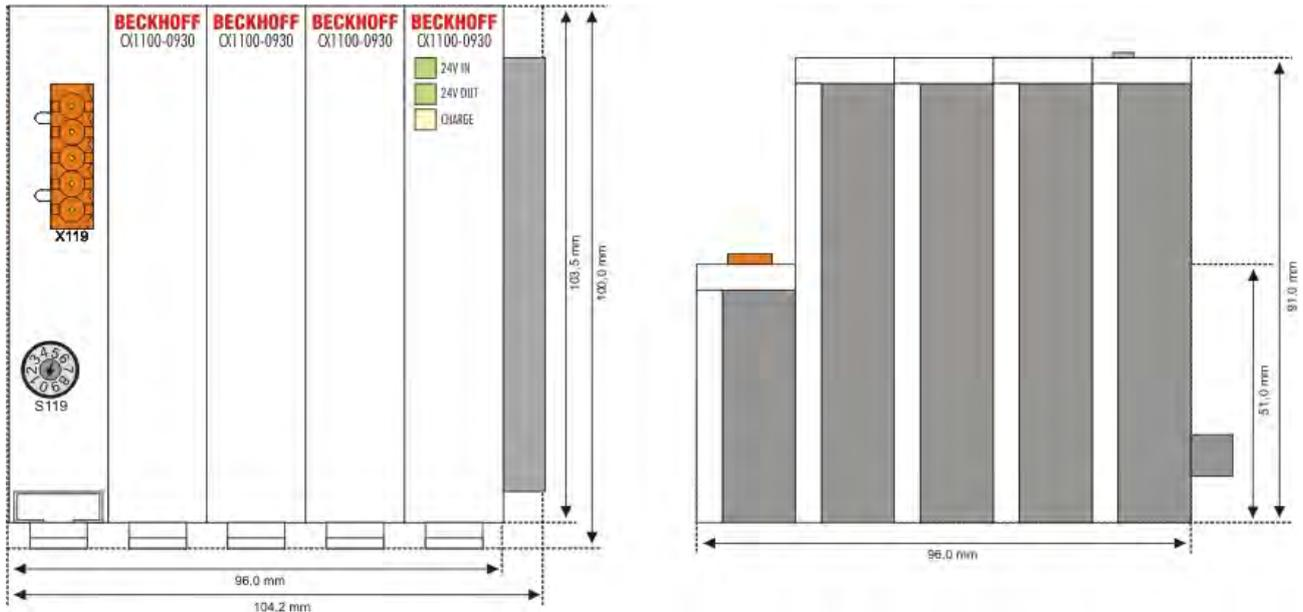
**4.1.2 Mechanical installation of the UPS Module**
