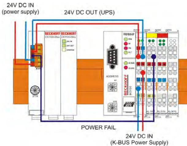
In case of power failure the UPS module rises the POWER-FAIL signal. The PLC program reads the input via the terminal bus and can shutdown the application. In this mode the control of the UPS module is controlled by the torque switch at the front side of the module.
