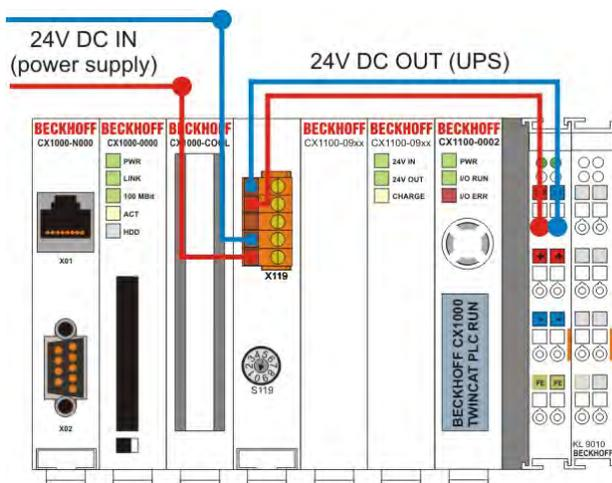
Though the power supply CX1100-0001 has no terminal bus interface the module is connected to the upper input connectors (24V). Older versions of the power supply are labeled with UPS -/+. These input are not used and more and must not be connected. The figure shows the correct connection.
