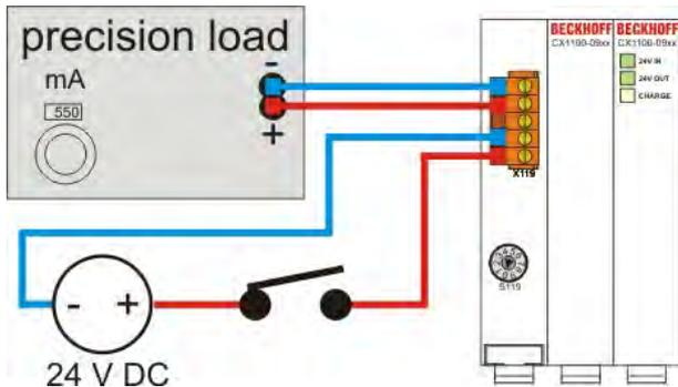
A measurement starts app. 30 seconds after the module signals full charge (CHARGE glows green). The power supply to the UPS is disconnected by releasing the switch. At the same time a clock is triggered. The measurement stops when the LEDs at the front of the module extinguish. Several series of measurements have been processed. The following diagrams show the retention time in relation to switch setting. As load the maximal load for the CX1100-0900 is used.
