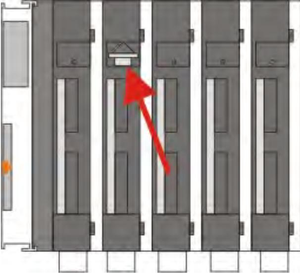
Only modules (CPU, fieldbus connections and UPS modules) that can be separated non-destructively feature a release device. Modules that cannot be separated only feature a marking point (with or without red paint seal). Applying force to these elements will destroy them.
