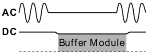
Fig. 2: Bridging power failures
