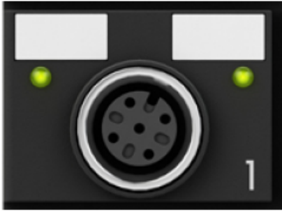
Fig. 7: IO-Link connection, master
