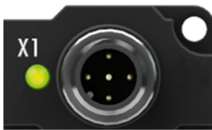
IO-Link Device status LED (narrow housing)
