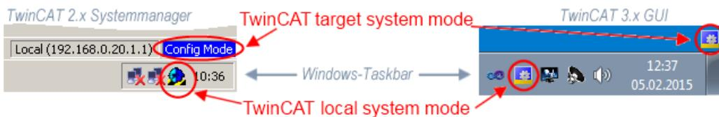
Fig. 64: Differentiation local/target system (left: TwinCAT 2; right: TwinCAT 3)
