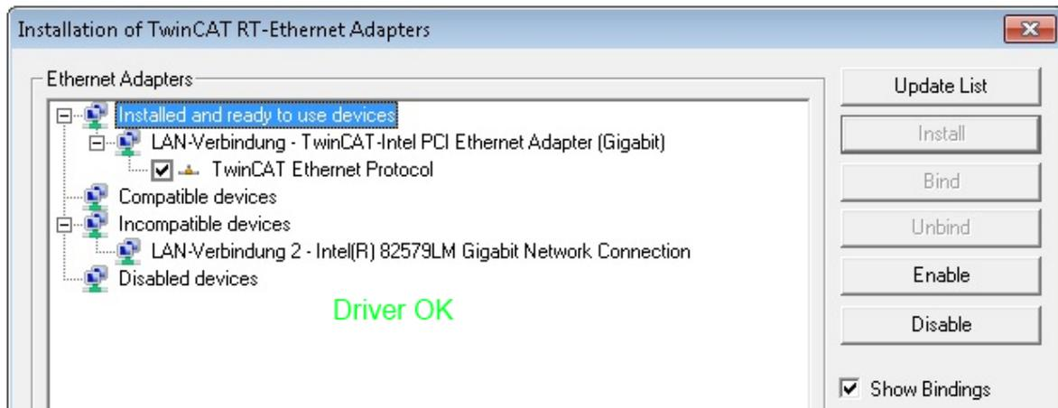
Fig. 45: Exemplary correct driver setting for the Ethernet port
