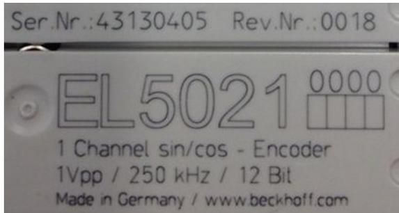
Fig. 1: EL5021 EL terminal, standard IP20 IO device with serial/ batch number and revision ID (since 2014/01)
