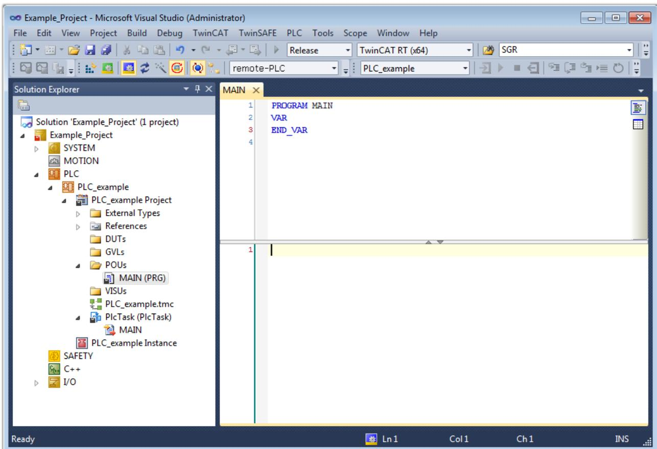
Fig. 51: Initial “Main” program of the standard PLC project
