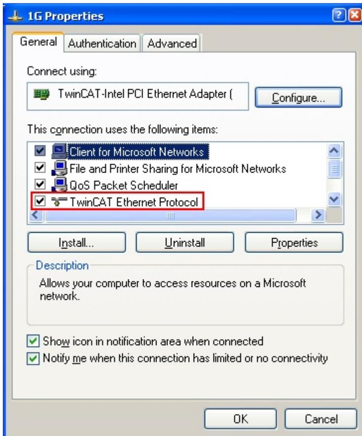
Fig. 67: Windows properties of the network interface
