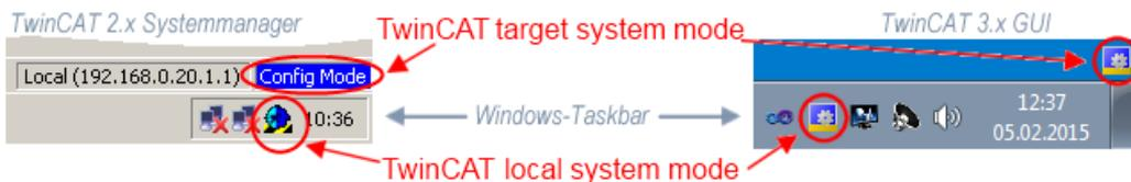
Fig. 89: Differentiation local/target system (left: TwinCAT 2; right: TwinCAT 3)
