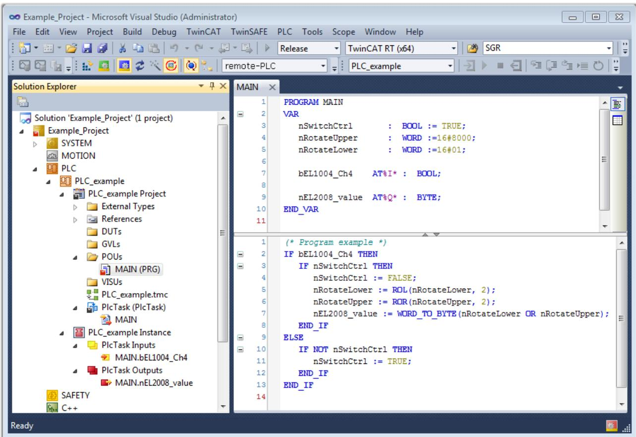
Fig. 52: Sample program with variables after a compile process (without variable integration)
