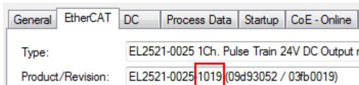
Fig. 95: Detection of EtherCAT terminal with revision -1019
