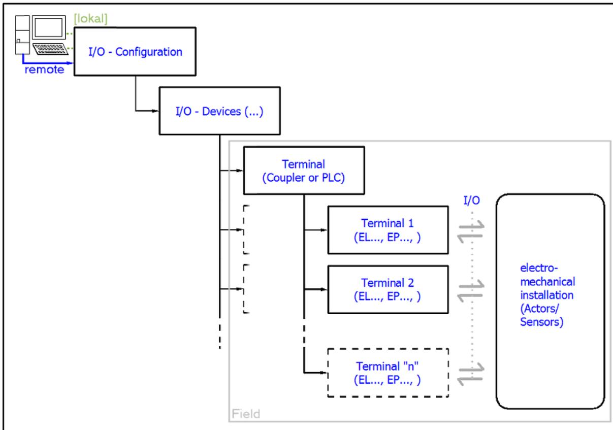
Fig. 21: Relationship between user side (commissioning) and installation
