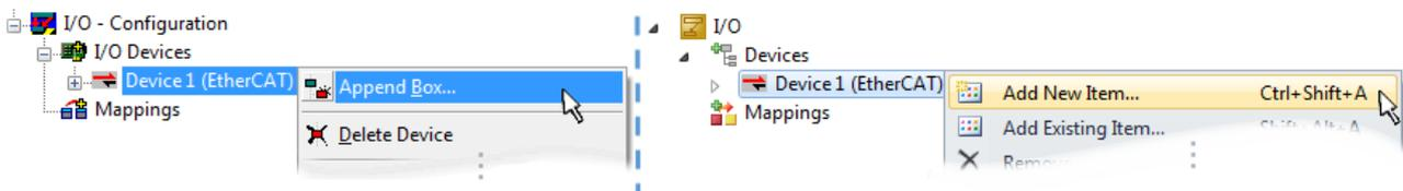
Fig. 83: Appending EtherCAT devices (left: TwinCAT 2; right: TwinCAT 3)
