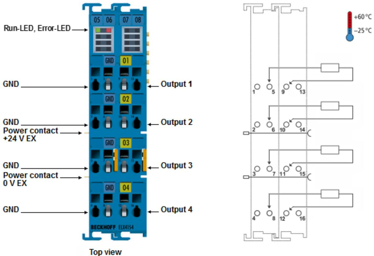
Fig. 4: ELX4154 - Four channel analog output terminal, 0/4...20 mA, single ended, 16 Bit, Ex i
