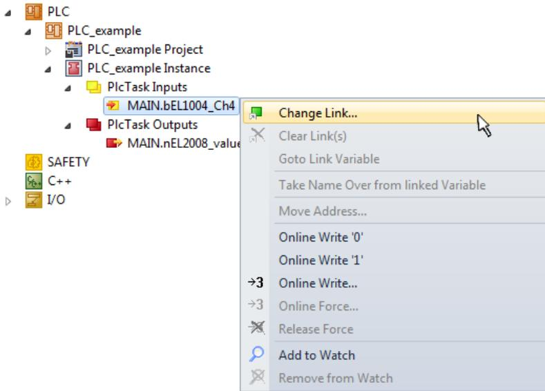
Fig. 54: Creating the links between PLC variables and process objects
