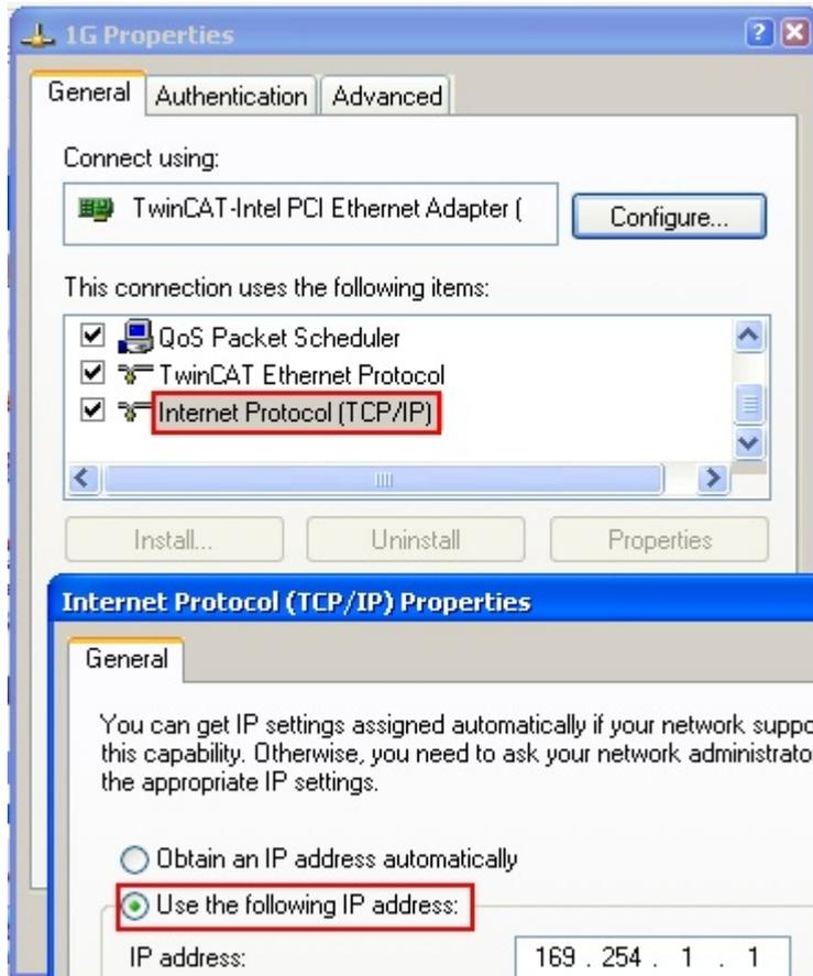
Fig. 70: TCP/IP setting for the Ethernet port
