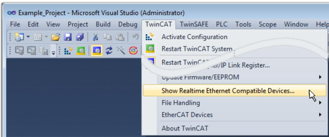
Fig. 64: Call up under VS Shell (TwinCAT 3)
