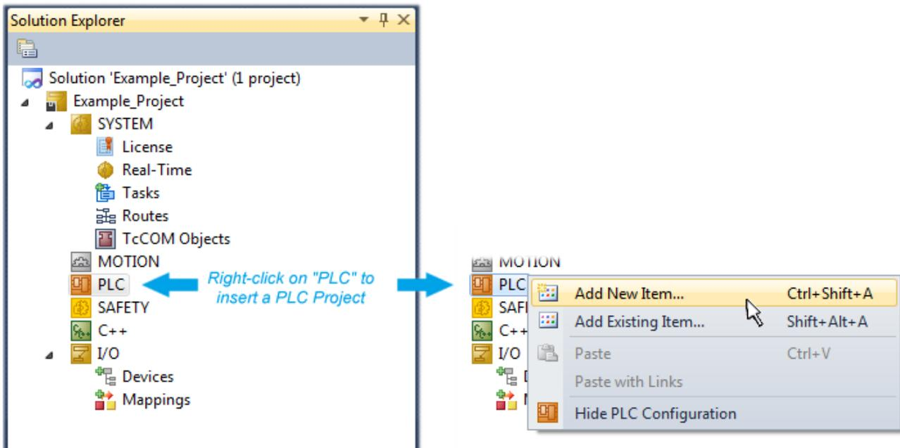
Fig. 49: Adding the programming environment in “PLC”
