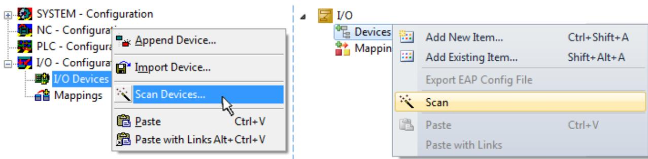
Fig. 90: Scan Devices (left: TwinCAT 2; right: TwinCAT 3)
