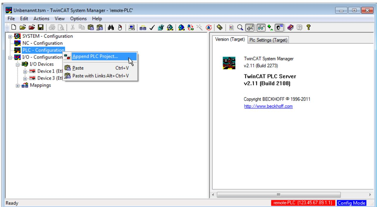
Fig. 32: Appending the TwinCAT PLC Control project
