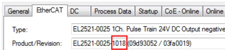
Fig. 94: Installing EthetCAT terminal with revision -1018
