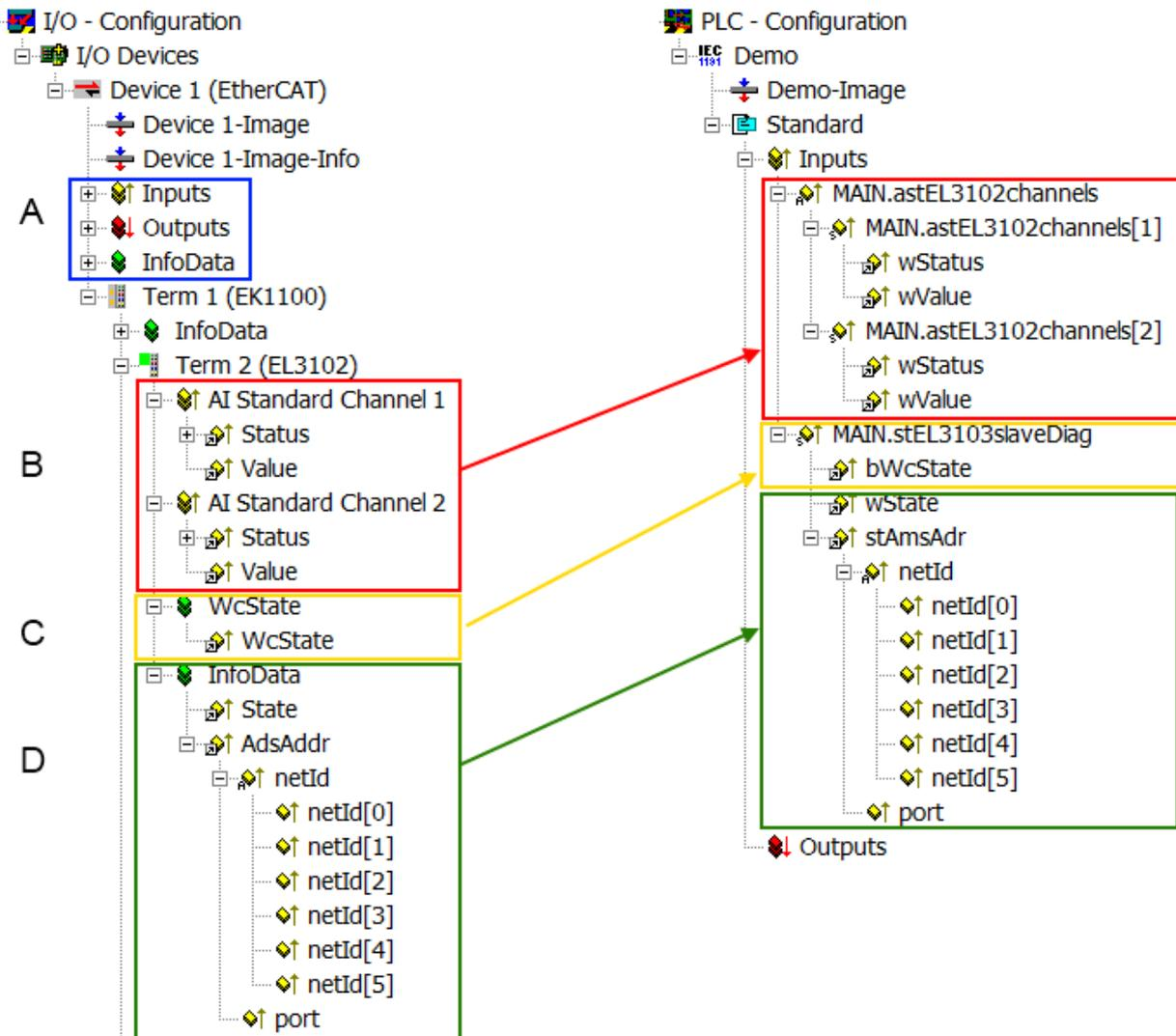
Fig. 121: Basic EtherCAT slave diagnosis in the PLC
