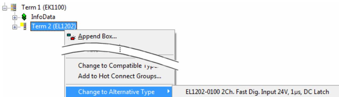
Fig. 109: TwinCAT 2 Dialog Change to Alternative Type
