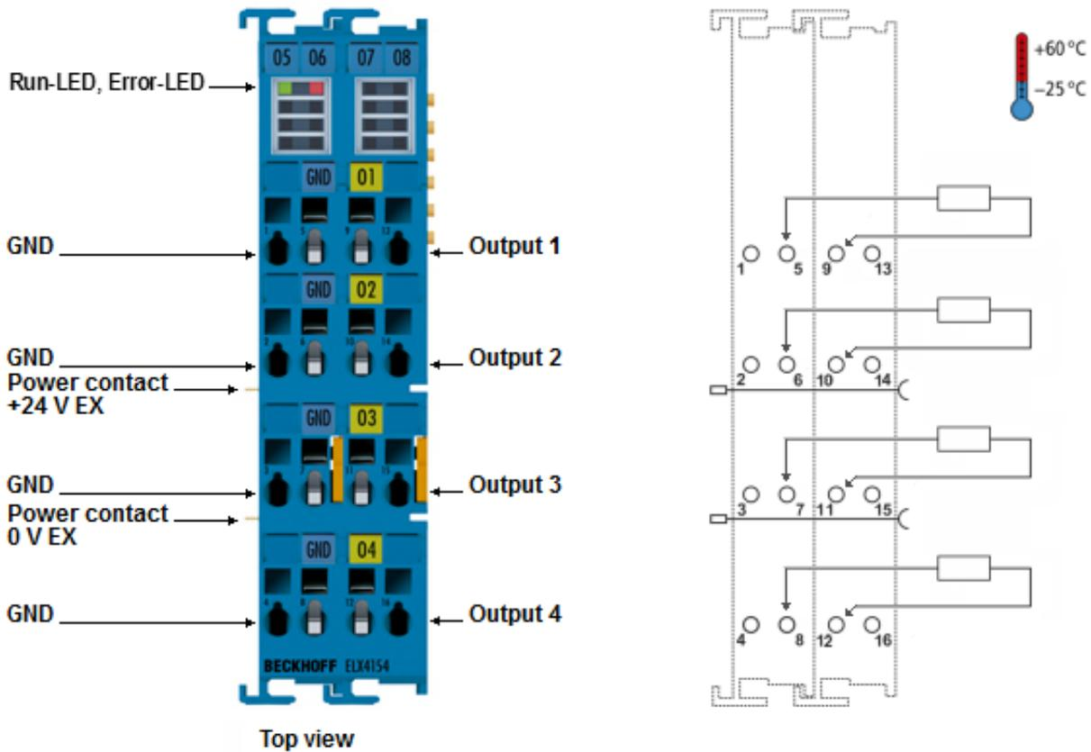
Fig. 20: ELX4154 - Contact assignment
