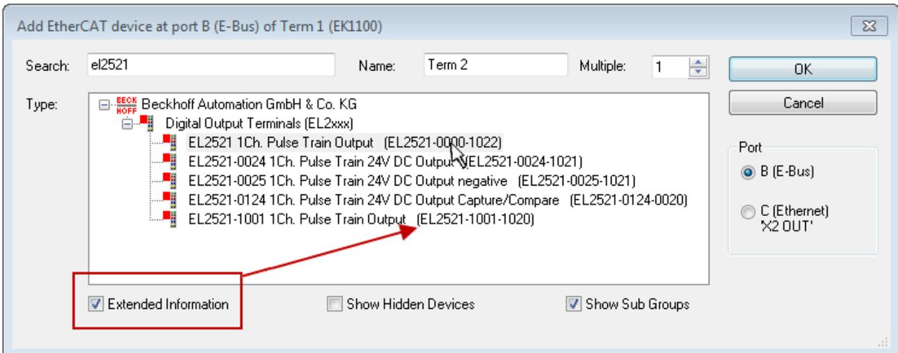
Fig. 85: Display of device revision
