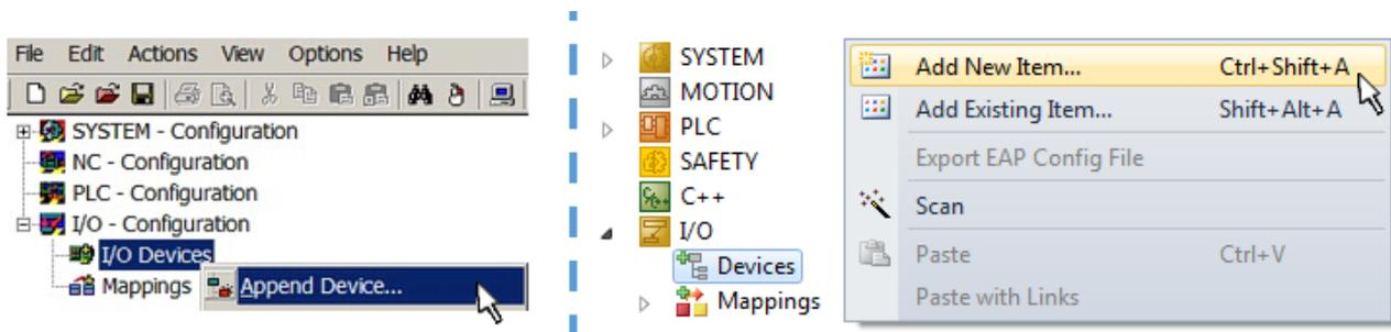
Fig. 79: Append EtherCAT device (left: TwinCAT 2; right: TwinCAT 3)
