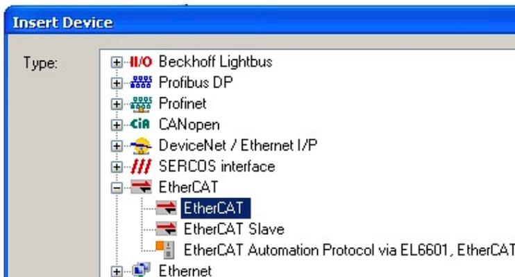
Fig. 80: Selecting the EtherCAT connection (TwinCAT 2.11, TwinCAT 3)
