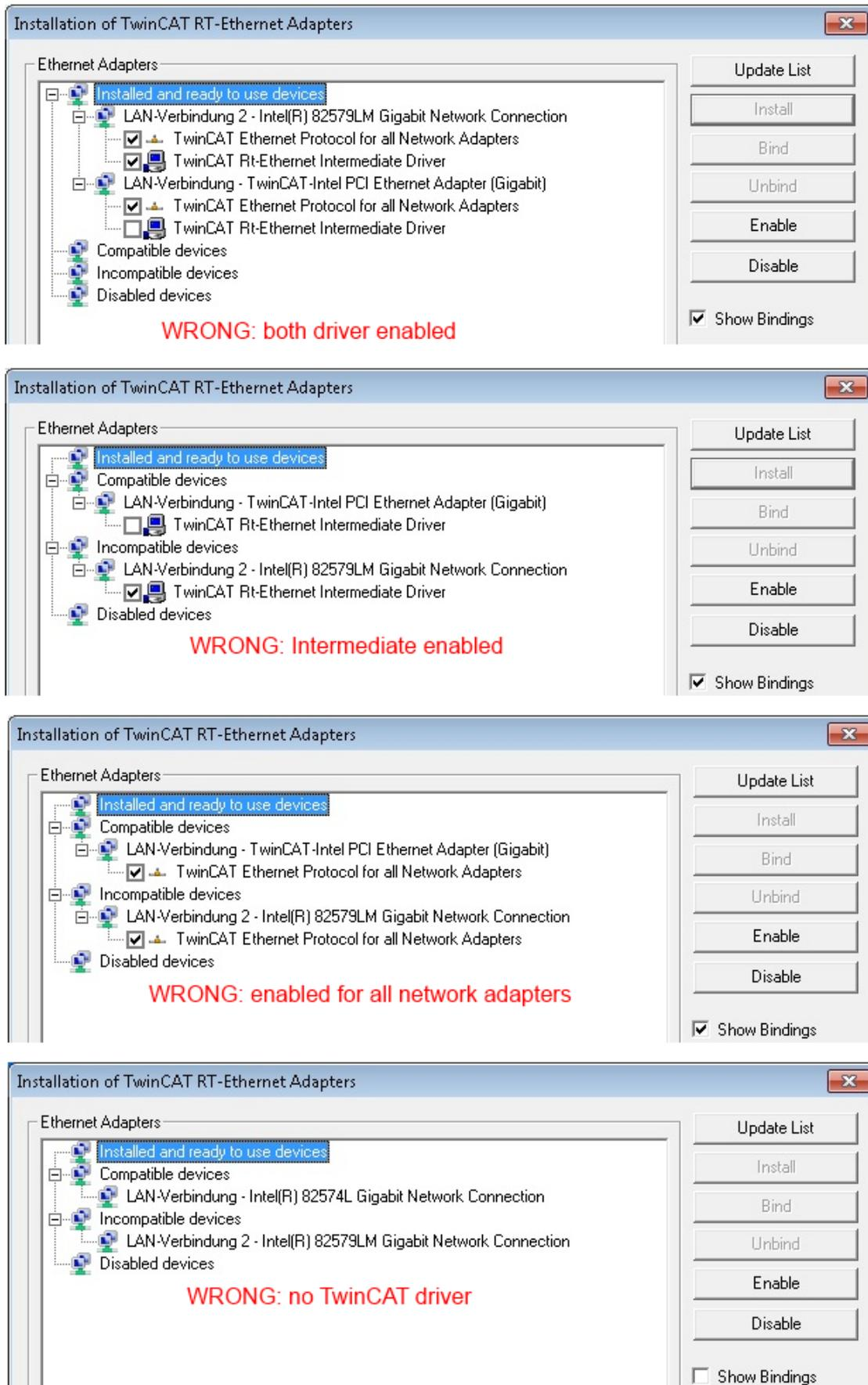
Fig. 69: Incorrect driver settings for the Ethernet port
