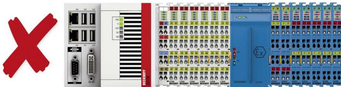
Fig. 13: Illegal arrangement - missing ELX9012 bus end cap.
