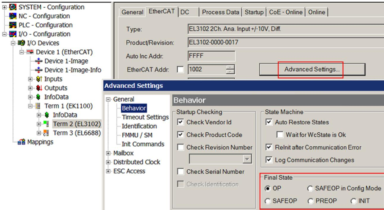
Fig. 125: Default target state in the Slave
