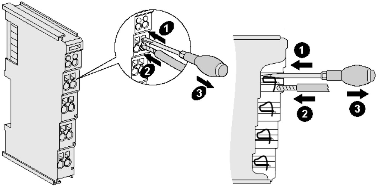
Fig. 19: Connecting a cable on a terminal point
