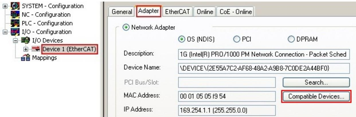
Fig. 66: EtherCAT device properties(TwinCAT 2): click on “Compatible Devices...” of tab “Adapte”
