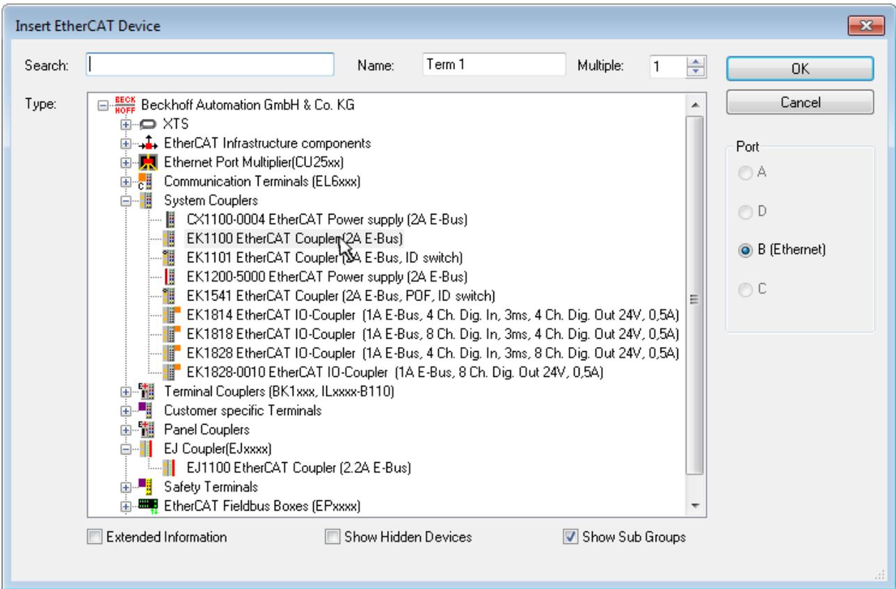
Fig. 84: Selection dialog for new EtherCAT device
