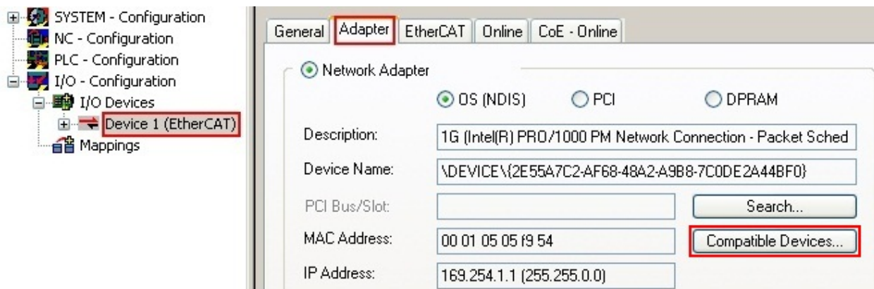
Fig. 76: EtherCAT device properties(TwinCAT 2): click on “Compatible Devices...” of tab “Adapte””
