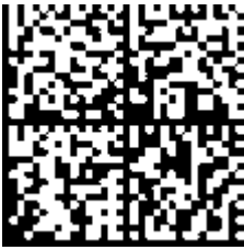
Fig. 3: Example DMC 1P072222SBTNk4p562d71KEL1809 Q1 51S678294
