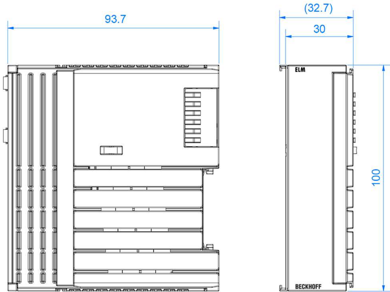
Fig. 128: Dimensions: ELM2xxx terminals
