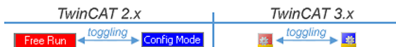
Fig. 102: Displaying of “Free Run” and “Config Mode” toggling right below in the status bar
