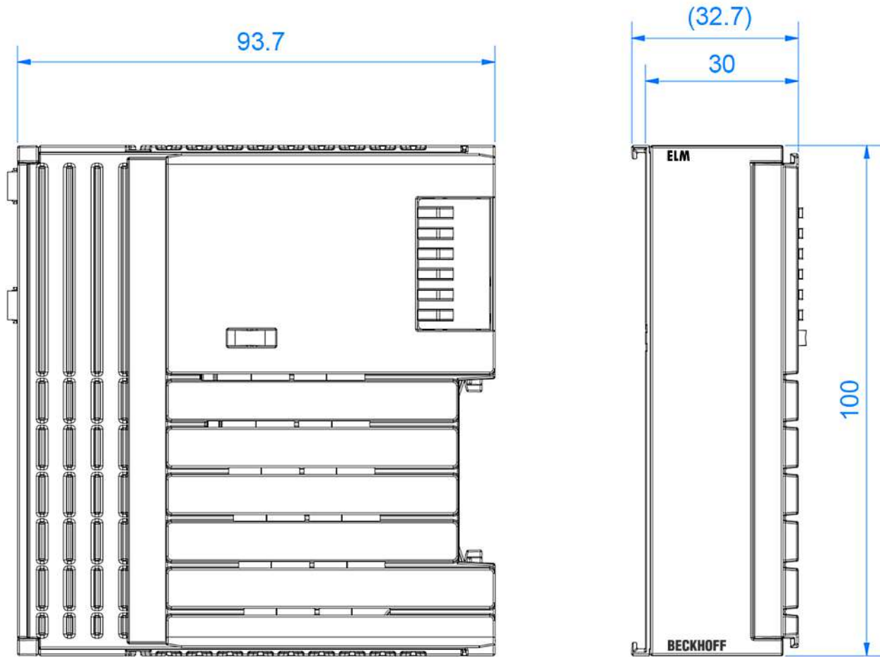
Fig. 129: Dimensions: ELM2xxx terminals
