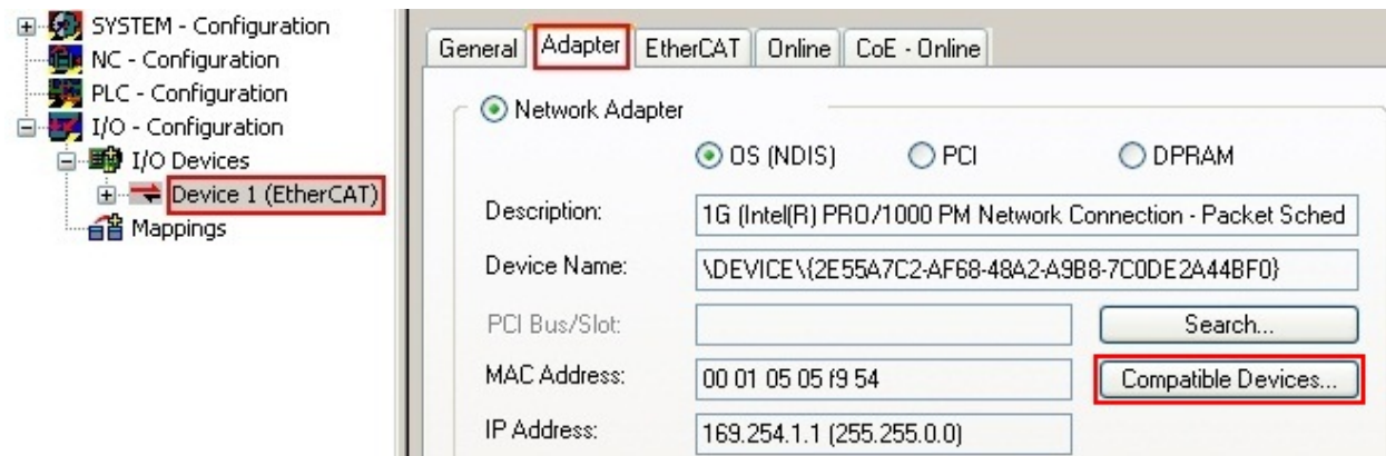
Fig. 78: EtherCAT device properties (TwinCAT 2): click on “Compatible Devices...” of tab “Adapter”
