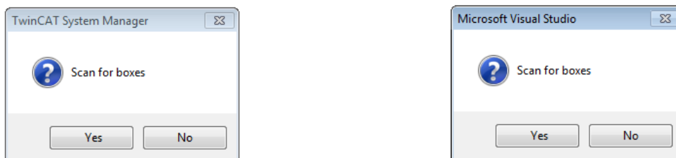
Fig. 104: Scan query after automatic creation of an EtherCAT device (left: TwinCAT 2; right: TwinCAT 3)
