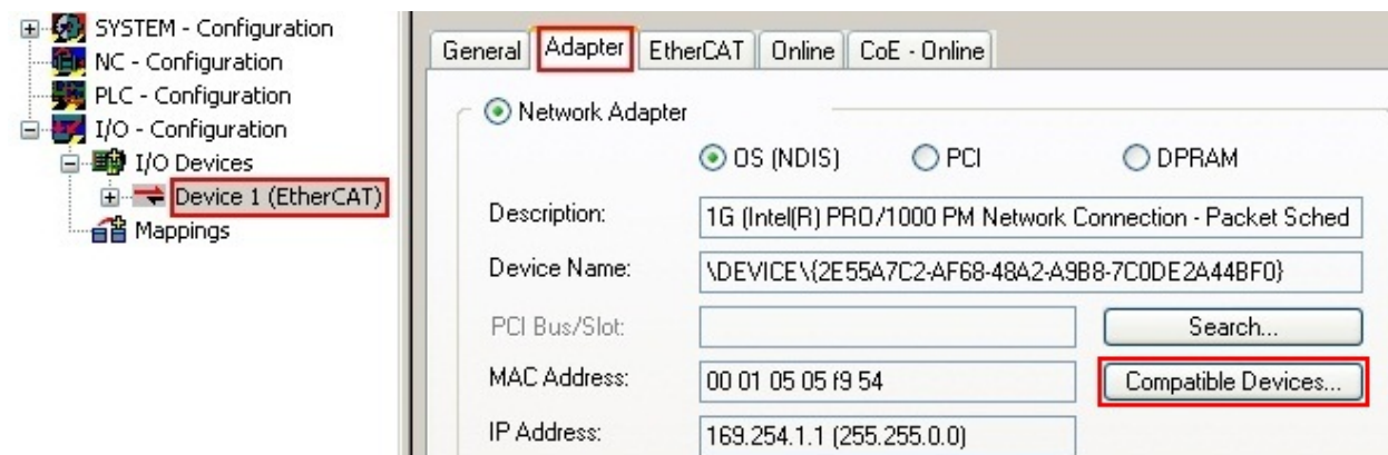
Fig. 69: EtherCAT device properties (TwinCAT 2): click on “Compatible Devices...” of tab “Adapter”
