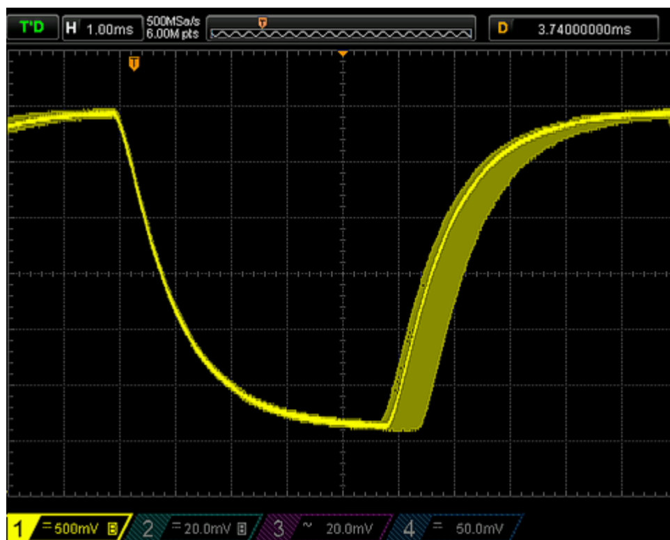
Fig. 148: EL4078 with 100 \mu s EtherCAT cycle time, output jitter > 1 ms
