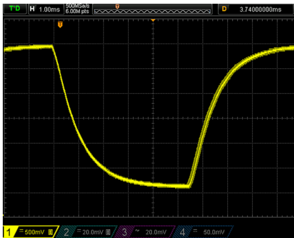
Fig. 147: EL4078 with 500 \mu s EtherCAT cycle time, output jitter according to theory \pm 0.5 cycles
