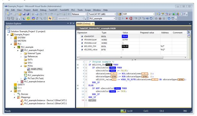
Fig. 91: TwinCAT development environment (VS shell): logged-in, after program startup
