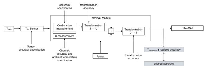
Fig. 25: Concatenation of the uncertainties in temperature measurement with thermocouples
