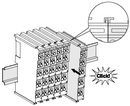
Fig. 37: Attaching on mounting rail
