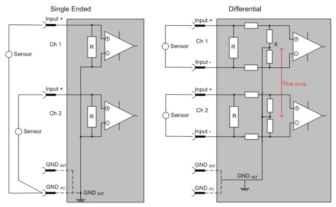
Fig. 183: SE and DIFF module as 2-channel version
