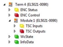
Fig. 159: TwinSAFE SC component process data, example EL5021-0090
