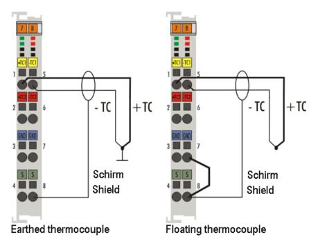
Fig. 44: Connection methods for earthed and earth-free thermocouples
