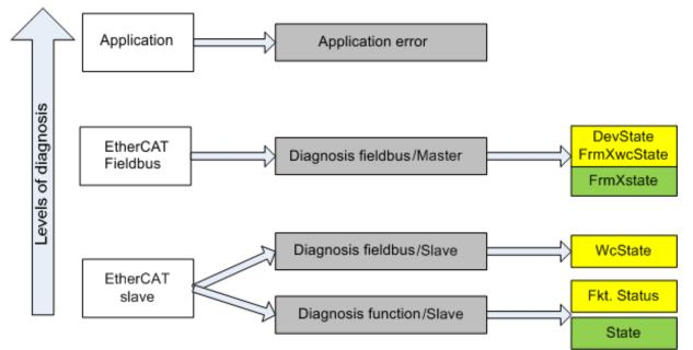
Fig. 149: Selection of the diagnostic information of an EtherCAT Slave
