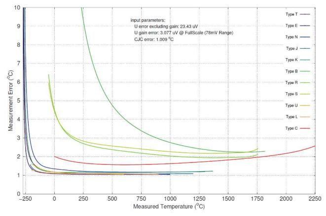
Fig. 26: Example of a thermocouple evaluation uncertainty analysis with an EL331x thermocouple terminal
