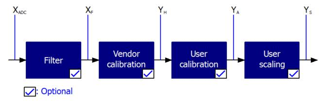
Fig. 171: Calculation of process data
