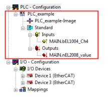
Fig. 62: PLC project integrated in the PLC configuration of the System Manager
