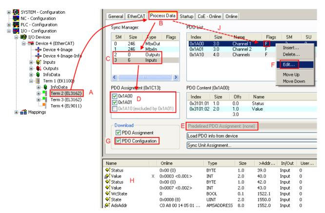
Fig. 143: Configuring the process data
