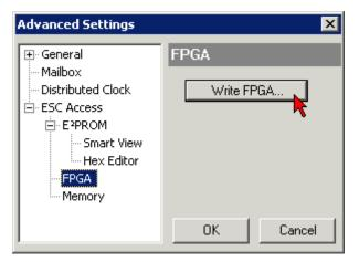
• Select the file (\*.rbf) with the new FPGA firmware, and transfer it to the EtherCAT device:
