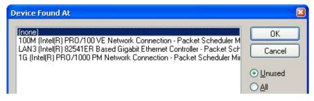
Fig. 110: Selecting the Ethernet port
