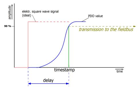
Fig. 190: Diagram signal delay (step response)
