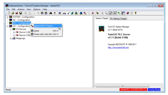
Fig. 61: Appending the TwinCAT PLC Control project
