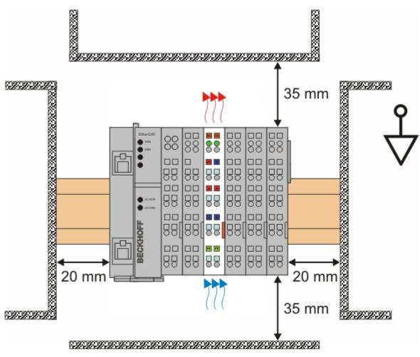
Fig. 49: Recommended distances for standard installation position
