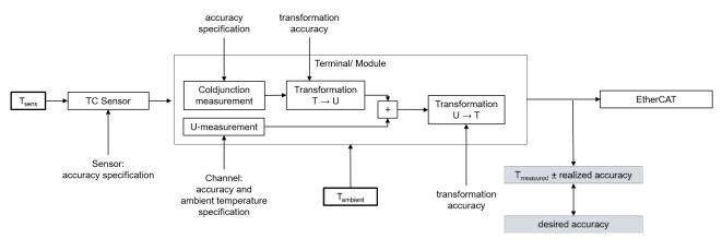
The given voltage specification is decisive for the achievable temperature measuring accuracy. It is applied to the possible thermocouple types in the following.
