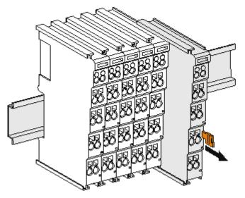
Fig. 38: Disassembling of terminal
