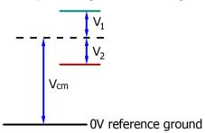
Fig. 187: Common-mode voltage (V<sub>cm</sub>)
