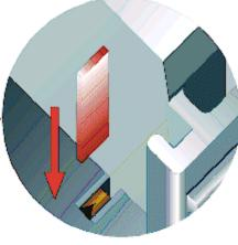
Fig. 39: Power contact on left side
