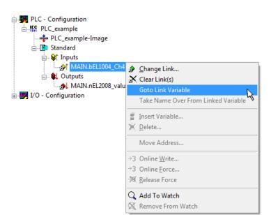
Fig. 66: Application of a "Goto Link" variable, using "MAIN.bEL1004\_Ch4" as a sample
