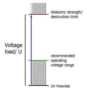
Fig. 188: Recommended operating voltage range
