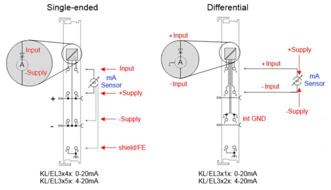
Fig. 185: Connection of externally supplied sensors
