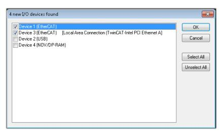
Fig. 75: Automatic detection of I/O devices: selection the devices to be integrated
