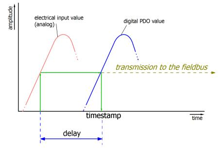
Fig. 191: Diagram signal delay (linear)
