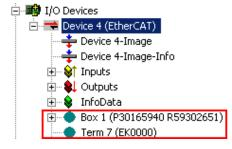
Fig. 132: Faulty identification
