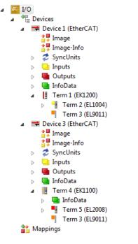
Fig. 76: Mapping of the configuration in VS shell of the TwinCAT3 environment
