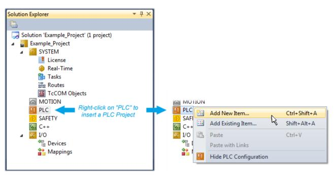
Fig. 78: Adding the programming environment in "PLC"
