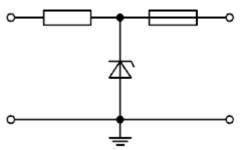
As already mentioned, these can influence the analog signal quality with respect to the above features, e.g. by temperature-dependent change of the internal resistance. Terms: Zener barrier
