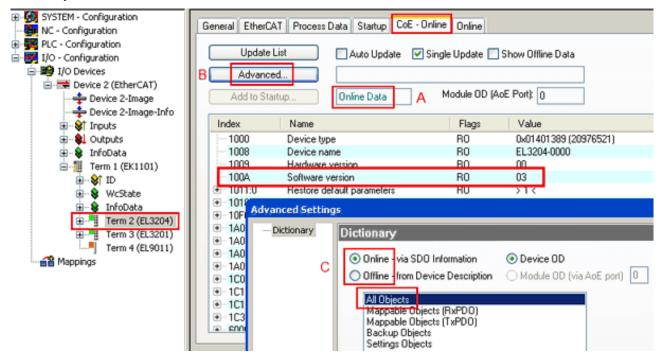
Fig. 201: Display of EL3204 firmware version
