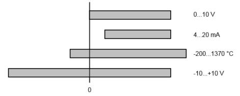
Fig. 182: Full scale value, measuring span
