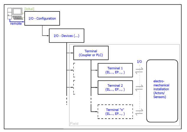
Fig. 50: Relationship between user side (commissioning) and installation
