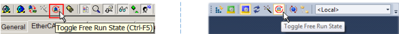
Fig. 112: TwinCAT can also be switched to this state by using a button (left: TwinCAT 2; right: TwinCAT 3)
