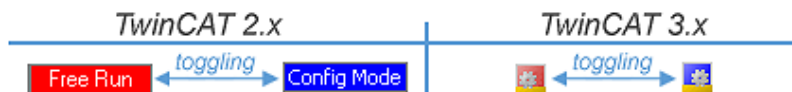
Fig. 182: Displaying of “Free Run” and “Config Mode” toggling right below in the status bar
