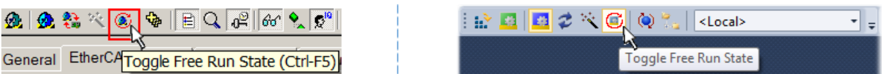
Fig. 154: TwinCAT can also be switched to this state by using a button (left: TwinCAT 2; right: TwinCAT 3)
