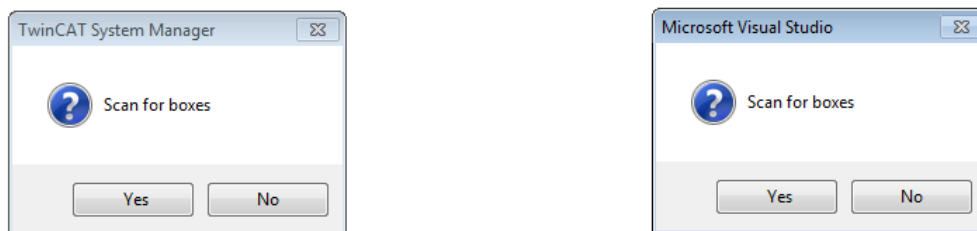
Fig. 99: Scan query after automatic creation of an EtherCAT device (left: TwinCAT 2; right: TwinCAT 3)
