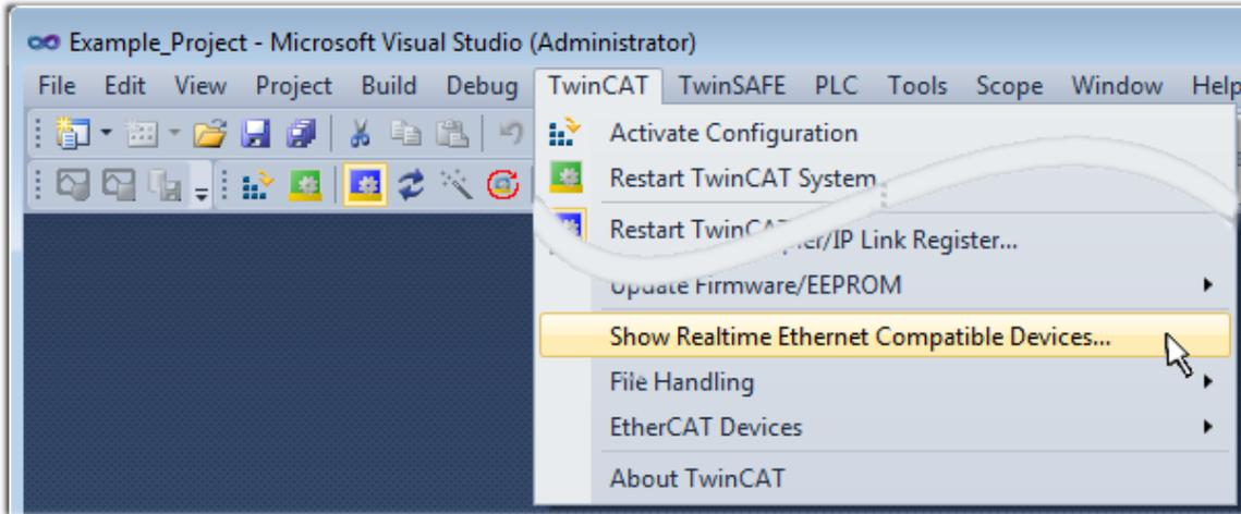
Abb. 28: Aufruf in VS Shell (TwinCAT 3)
