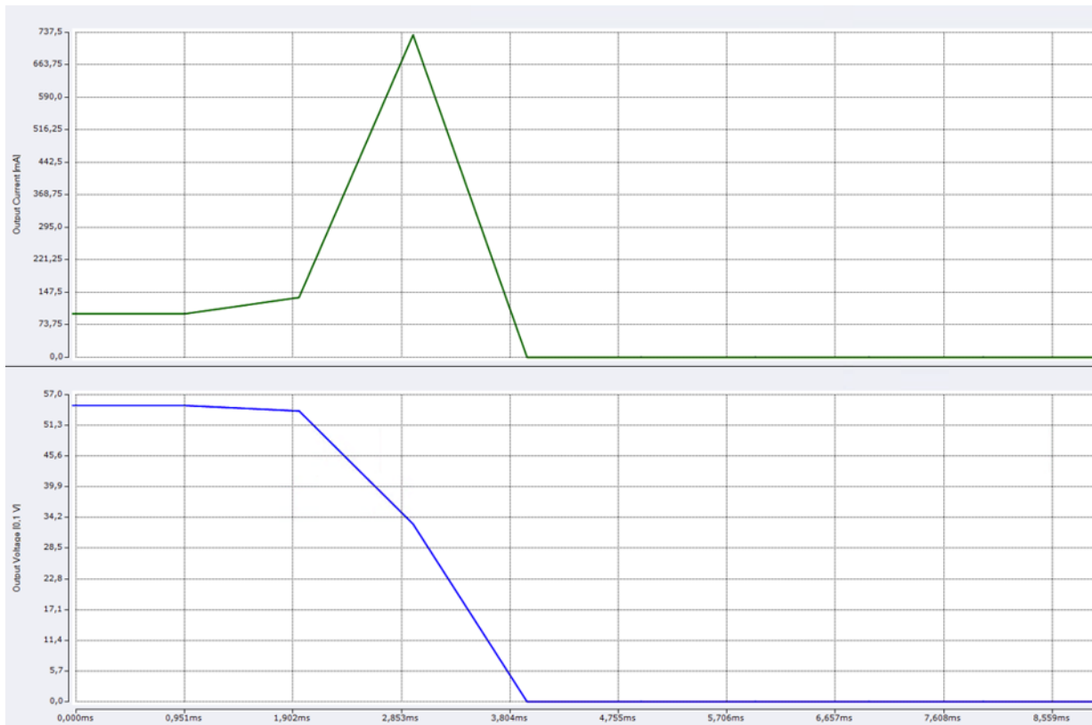
Fig. 235: Time for detection of a short-circuit
