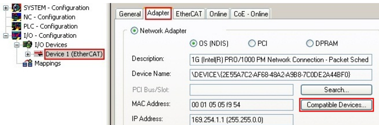
Fig. 76: EtherCAT device properties (TwinCAT 2): click on “Compatible Devices...” of tab “Adapter”
