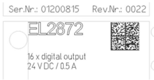
Fig. 1: EL2872 with revision 0022 and serial number 01200815
