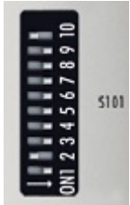
Abb. 15: DIP-Schalter S001: links off "0", rechts on "1"
