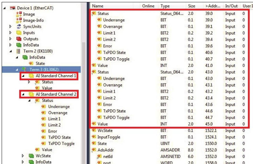
Fig. 22: Meaning of the individual bits with all subvariables and structure contents for the EL3062.
