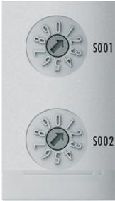
Fig. 16: Address selection switches of the EK3100.
