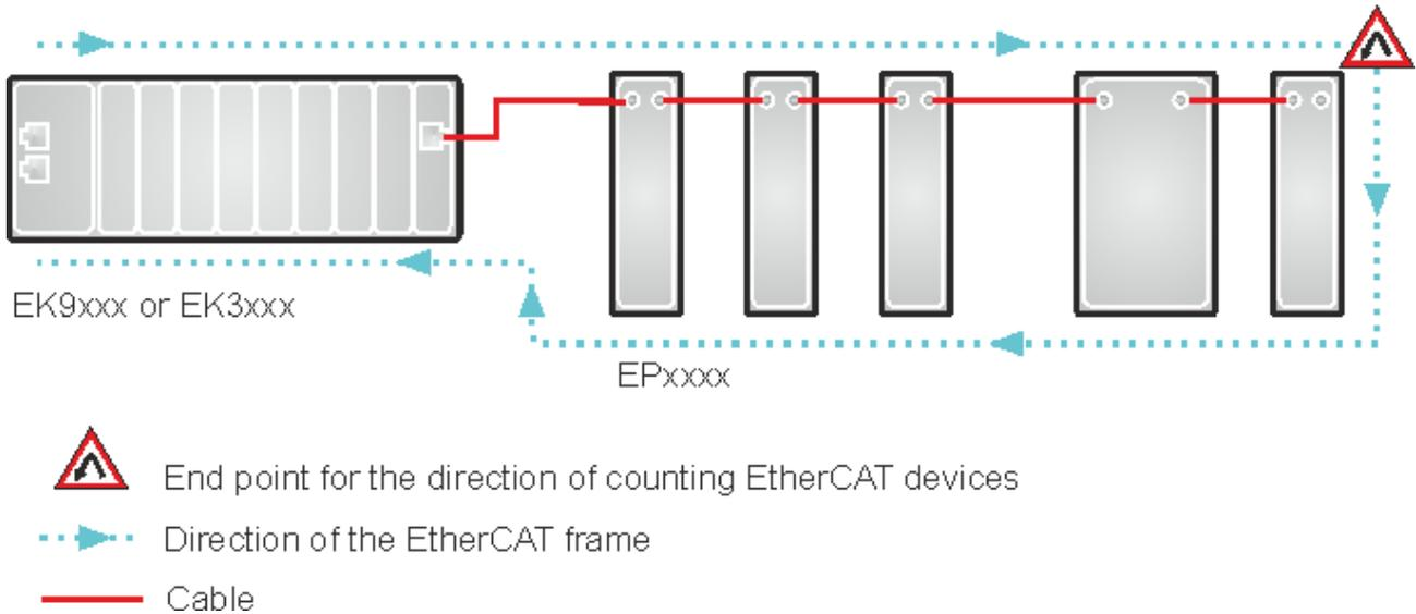
Fig. 19: Sample configuration with EPxxxx EtherCAT Box
