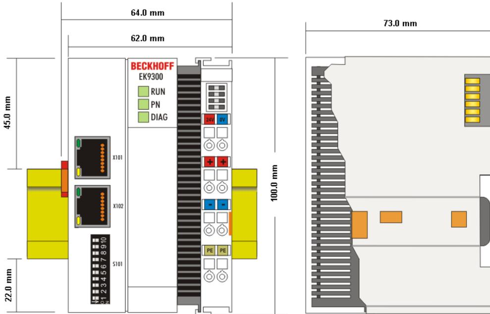
Fig. 7: Dimensions, based on EK9300 as an example.
