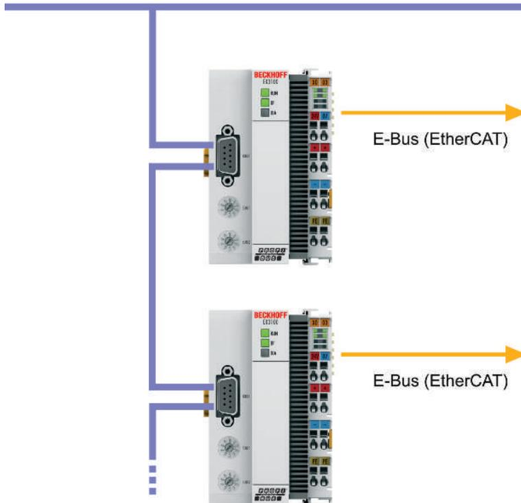
Fig. 14: PROFIBUS topology with the EK3100 Bus Coupler.
