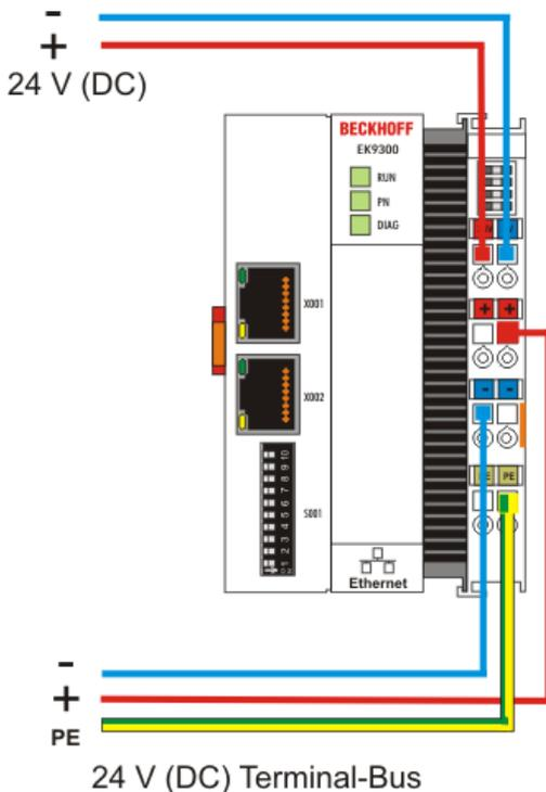
Fig. 11: Bus Coupler power supply, based on the EK9300 as an example.
