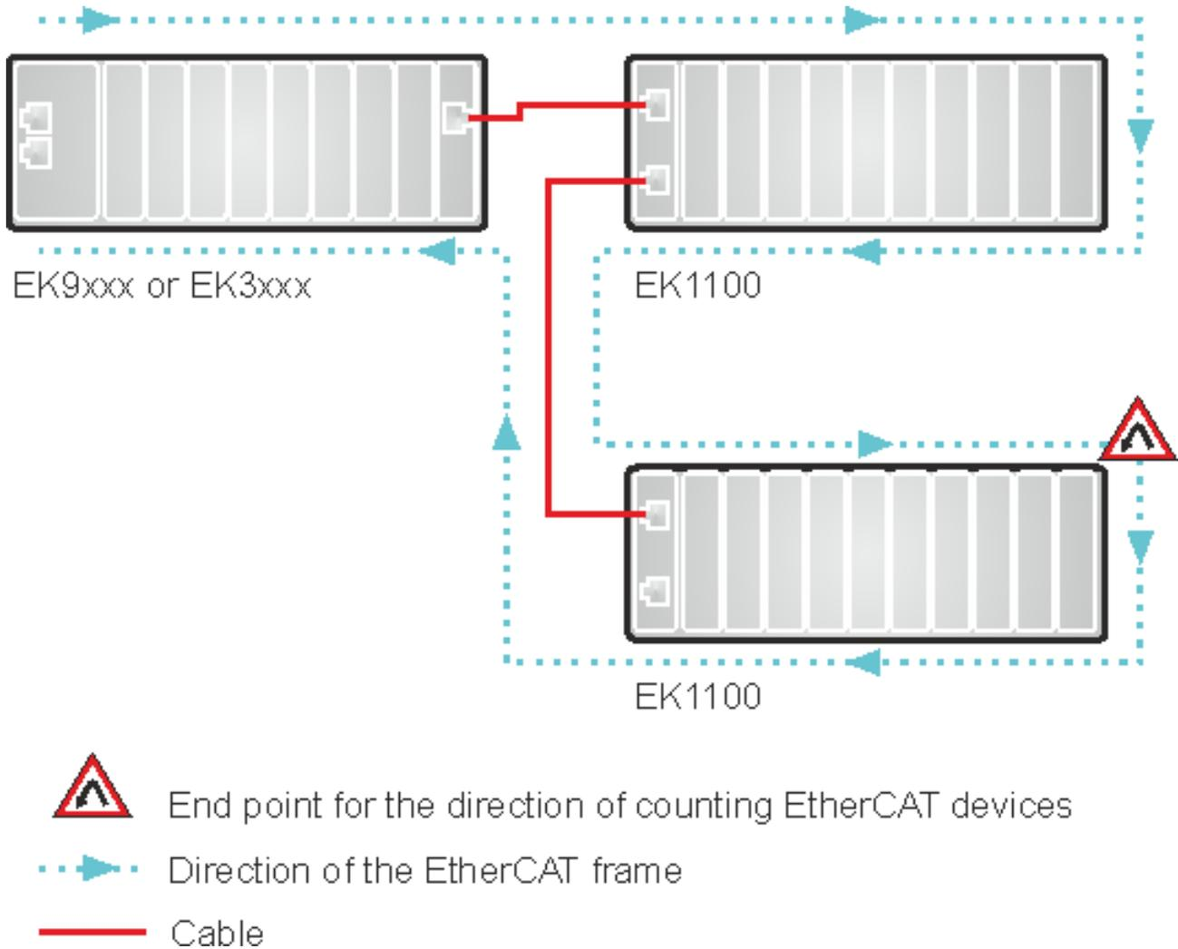
Fig. 18: Sample configuration with EK1100 EtherCAT coupler
