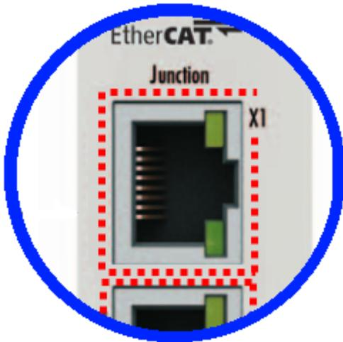
Abb. 5: Fast-Hot-Connect Ports des EK1122-0080
