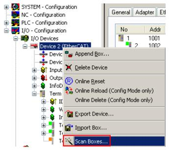
Fig. 28: Scan the subordinate field by right-clicking on the EtherCAT device
