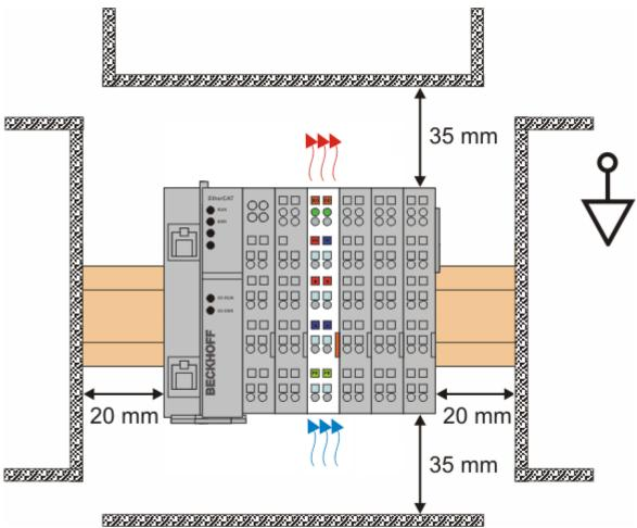
Fig. 9: Recommended distances for standard installation position
