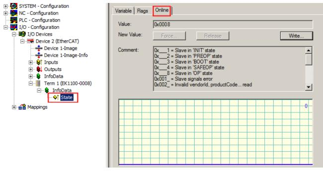
Fig. 26: TwinCAT tree showing the EK1100-0008 as an example, State tab online
