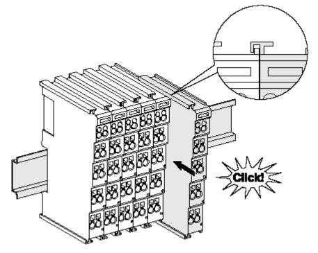
Fig. 12: Installation on the mounting rail
