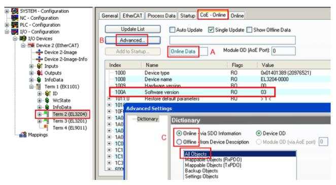
Fig. 33: Display of EL3204 firmware version
