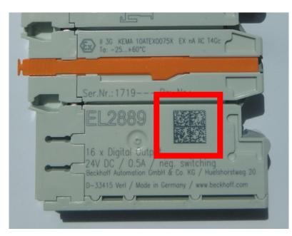
Fig. 2: BIC as data matrix code (DMC, code scheme ECC200)
