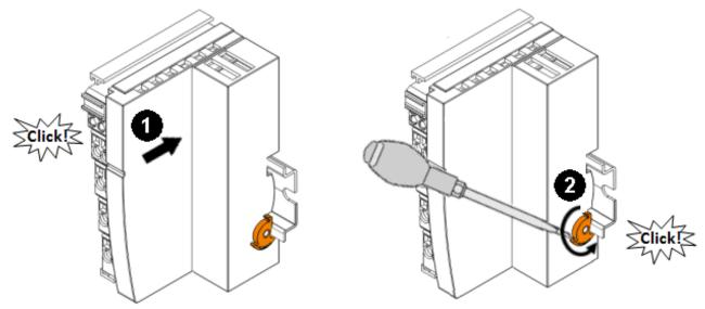
Fig. 11: Mounting the EtherCAT EJ Coupler on the mounting rail of the signal distribution board
