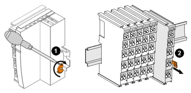
Fig. 13: Disassembly from the mounting rail
