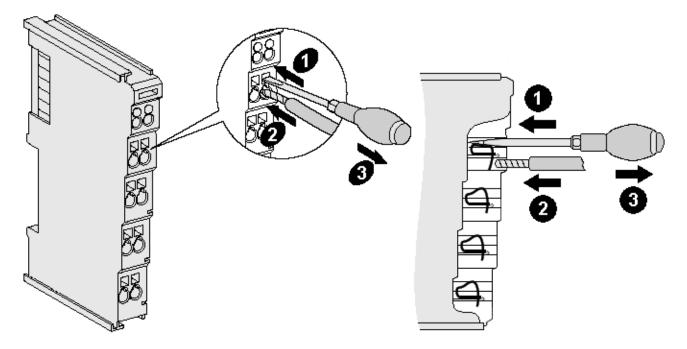
Fig. 18: Connecting a cable on a terminal point
