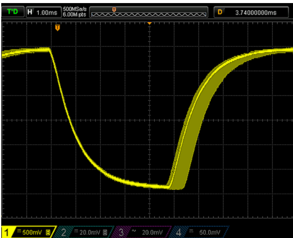
Fig. 28: EL4078 with 100 \mu s EtherCAT cycle time, output jitter > 1 ms
