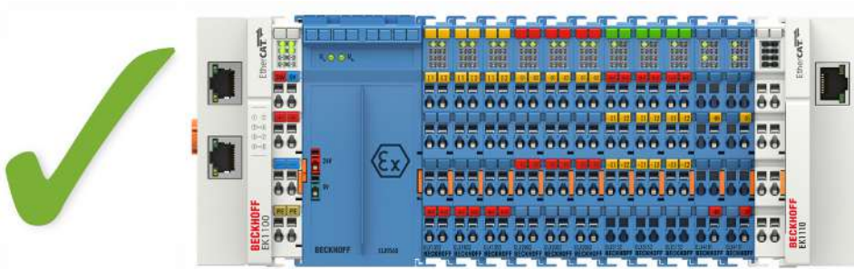
Fig. 9: Permitted arrangement - terminals that do not belong to the ELX series are placed before and after the ELX terminal segment. Isolation is provided by the ELX9560 at the beginning of the ELX terminal segment and the EK1110 at the end of the ELX terminal segment.
