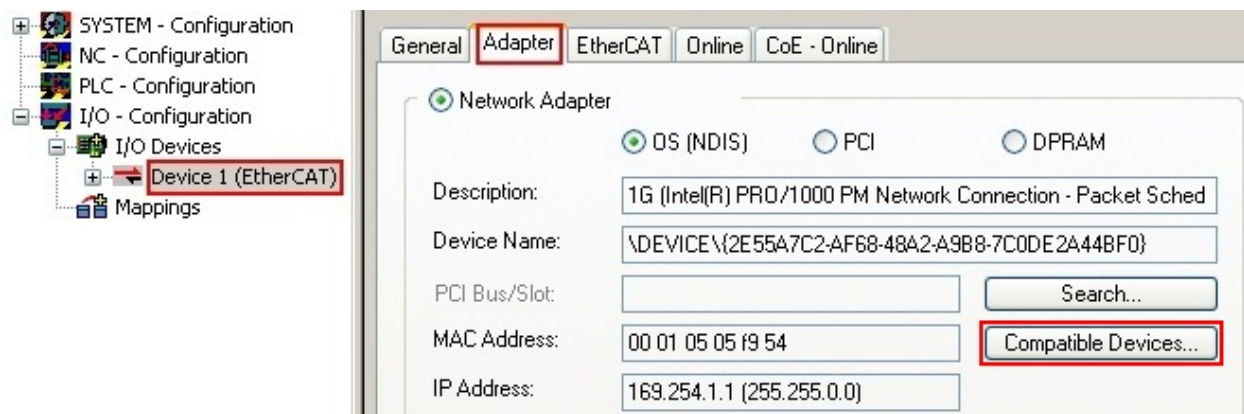
Fig. 87: EtherCAT device properties(TwinCAT 2): click on “Compatible Devices...” of tab “Adapte”
