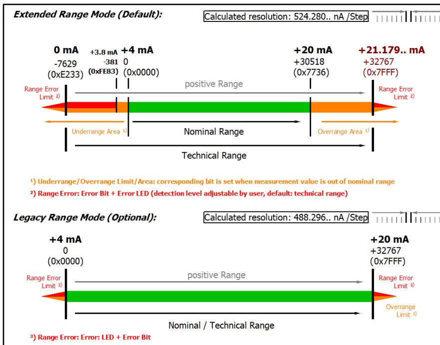
Technical note: The detection level for underrange and range error of 0 value area is located at 3.8 mA (-1% of the FSV full scale vale). This has been configured to prevent a misleading setting of the error bit.
