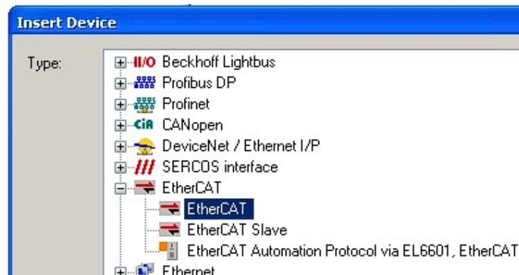
附图 91: 选择EtherCAT连接 (TwinCAT 2.11, TwinCAT 3)
