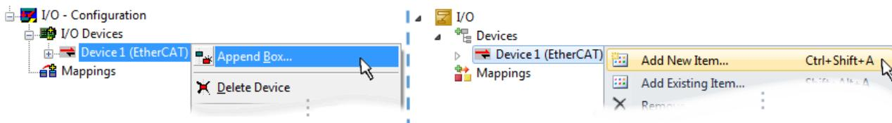
附图 94: 添加EtherCAT设备 (左: TwinCAT 2; 右: TwinCAT 3)
