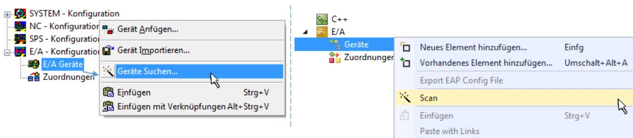
Abb. 95: Scan Devices (links: TwinCAT 2; rechts: TwinCAT 3)
