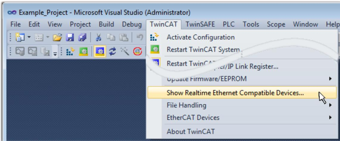
Fig. 67: Call up under VS Shell (TwinCAT 3)
