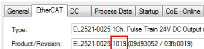
Fig. 99: Detection of EtherCAT terminal with revision -1019
