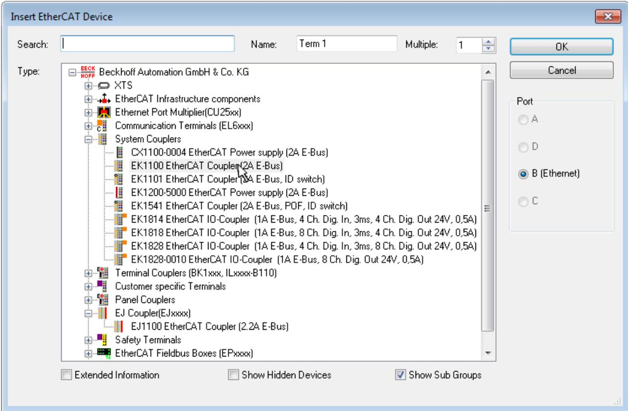
Fig. 88: Selection dialog for new EtherCAT device
