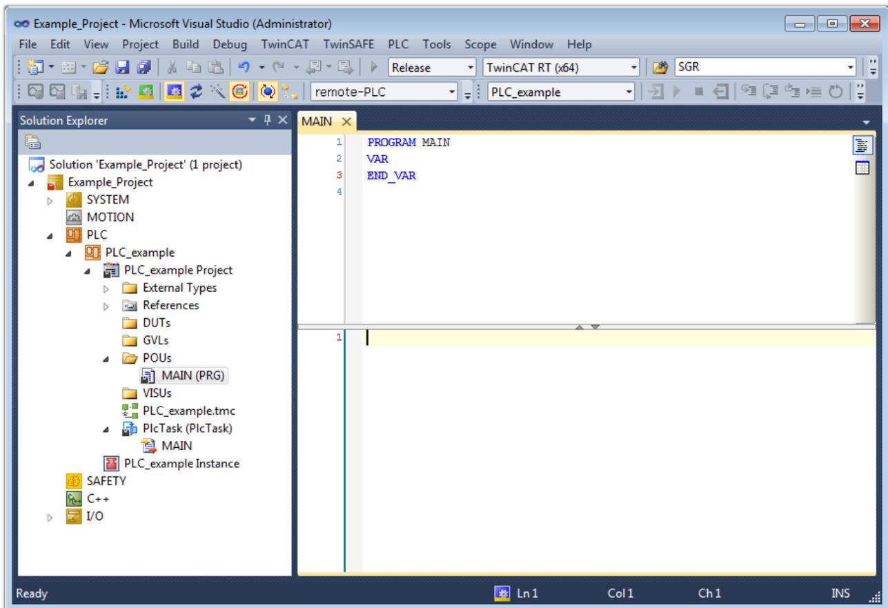
Fig. 54: Initial “Main” program for the standard PLC project
