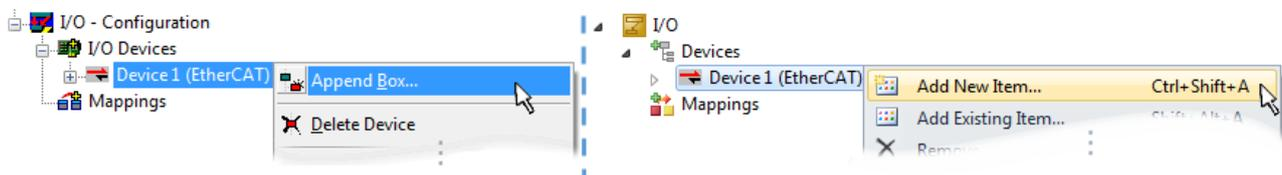
Fig. 87: Appending EtherCAT devices (left: TwinCAT 2; right: TwinCAT 3)
