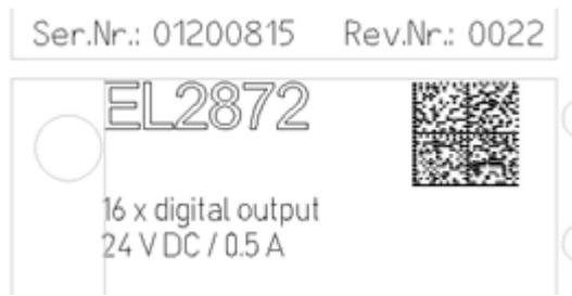
Fig. 1: EL2872 with revision 0022 and serial number 01200815
