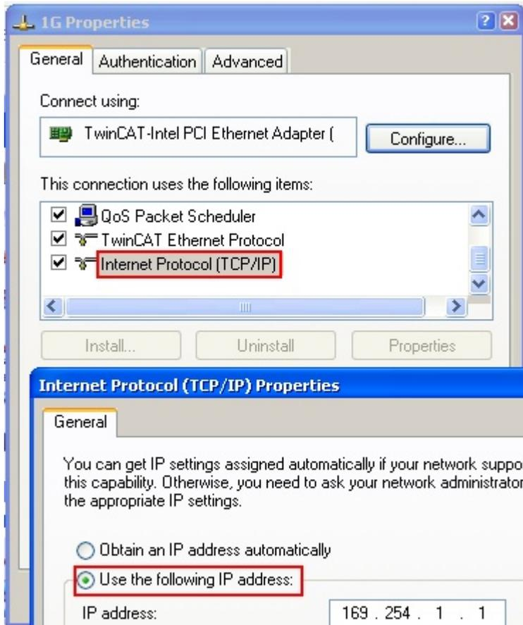
Fig. 74: TCP/IP setting for the Ethernet port
