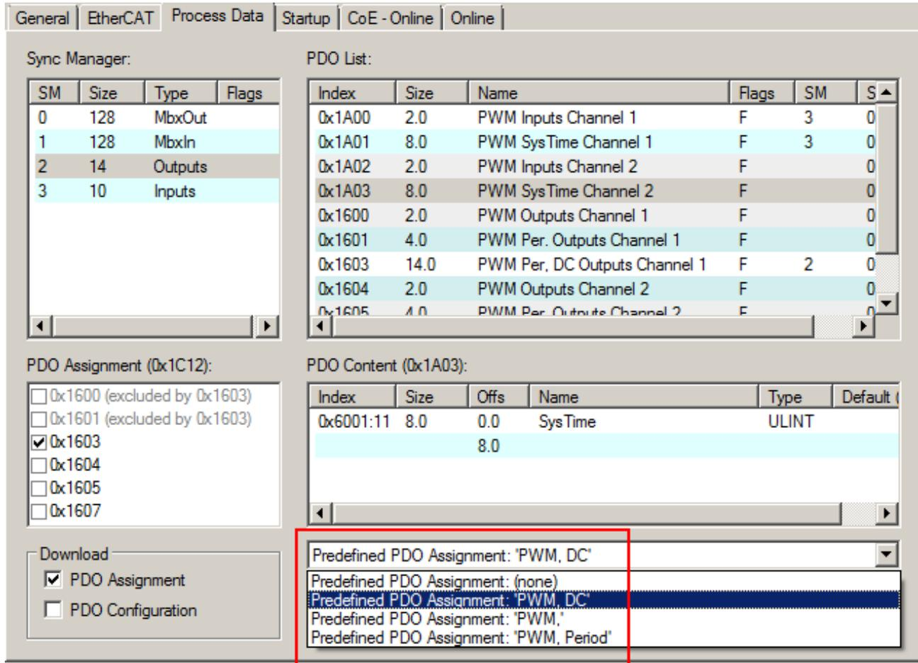
Fig. 133: EL2502-0010 - selection of the process data via Predefined PDO Assignment
