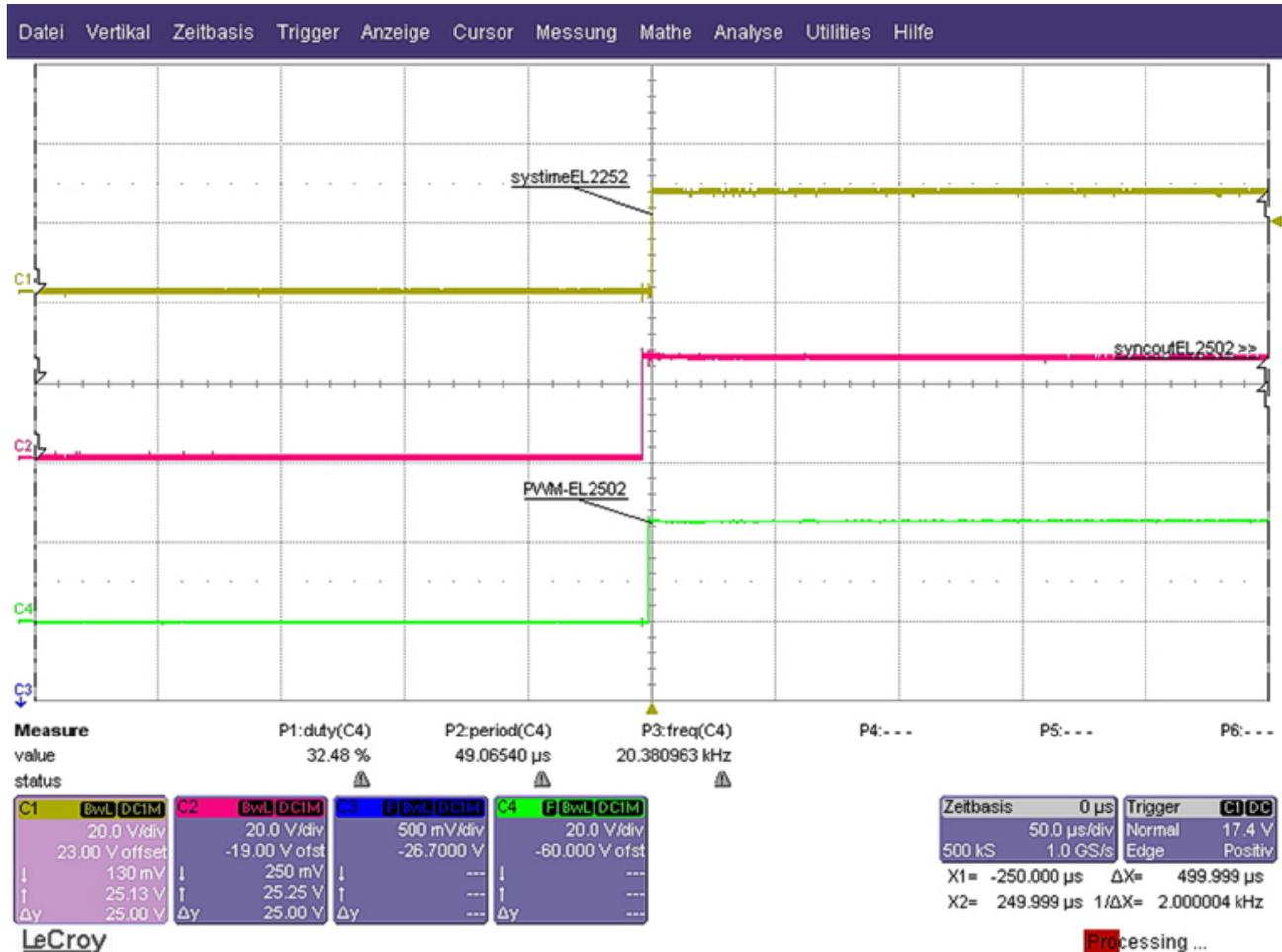
Fig. 138: Diagram „Immediate = TRUE”, duty factor 0 to 100%
