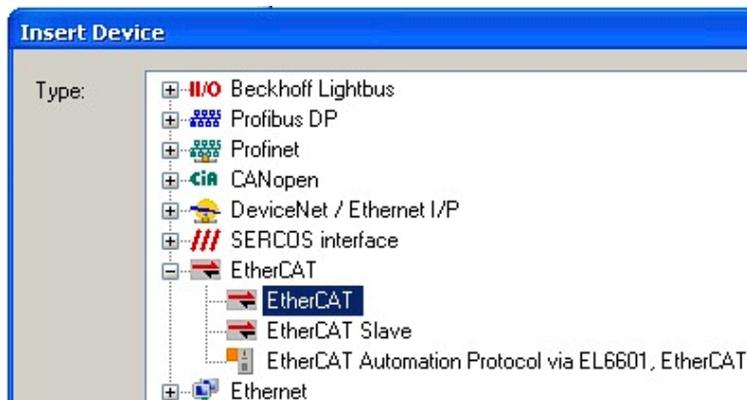
Fig. 84: Selecting the EtherCAT connection (TwinCAT 2.11, TwinCAT 3)
