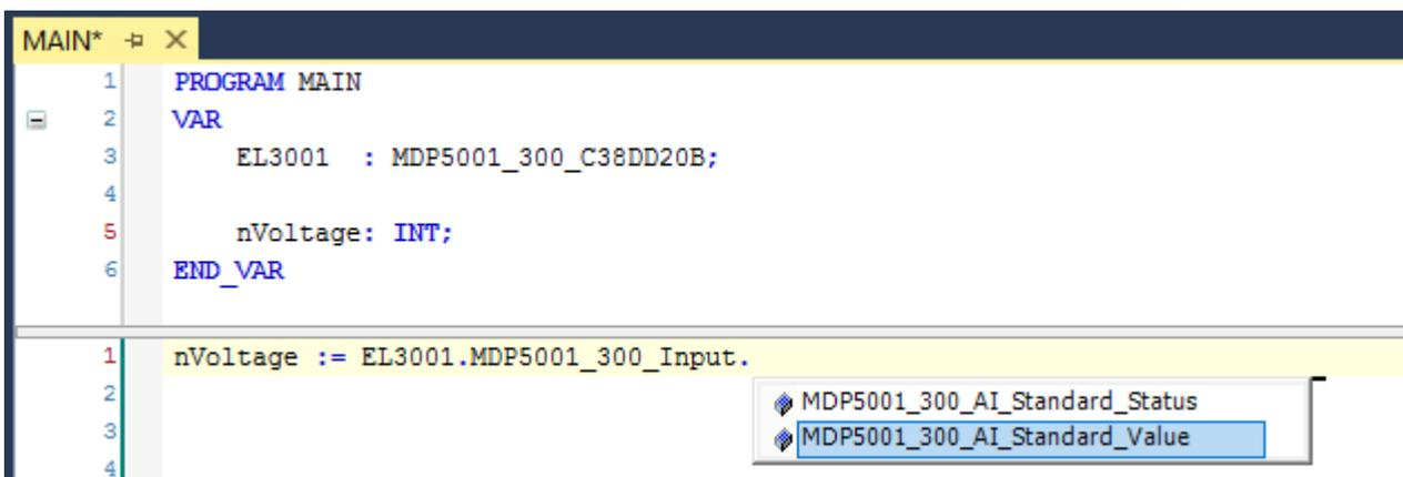
Fig. 64: Reading a variable from the structure of the process data
