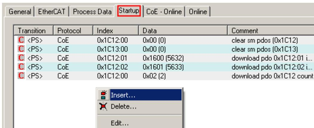
Fig. 9: Startup list in the TwinCAT System Manager
