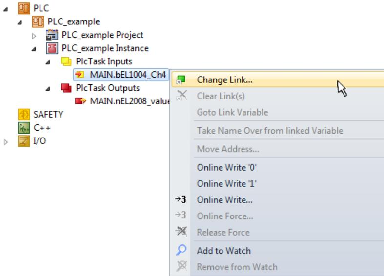
Fig. 57: Creating the links between PLC variables and process objects
