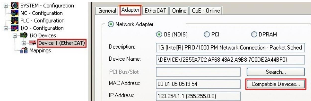
Fig. 70: EtherCAT device properties (TwinCAT 2): click on “Compatible Devices...” of tab “Adapter”
