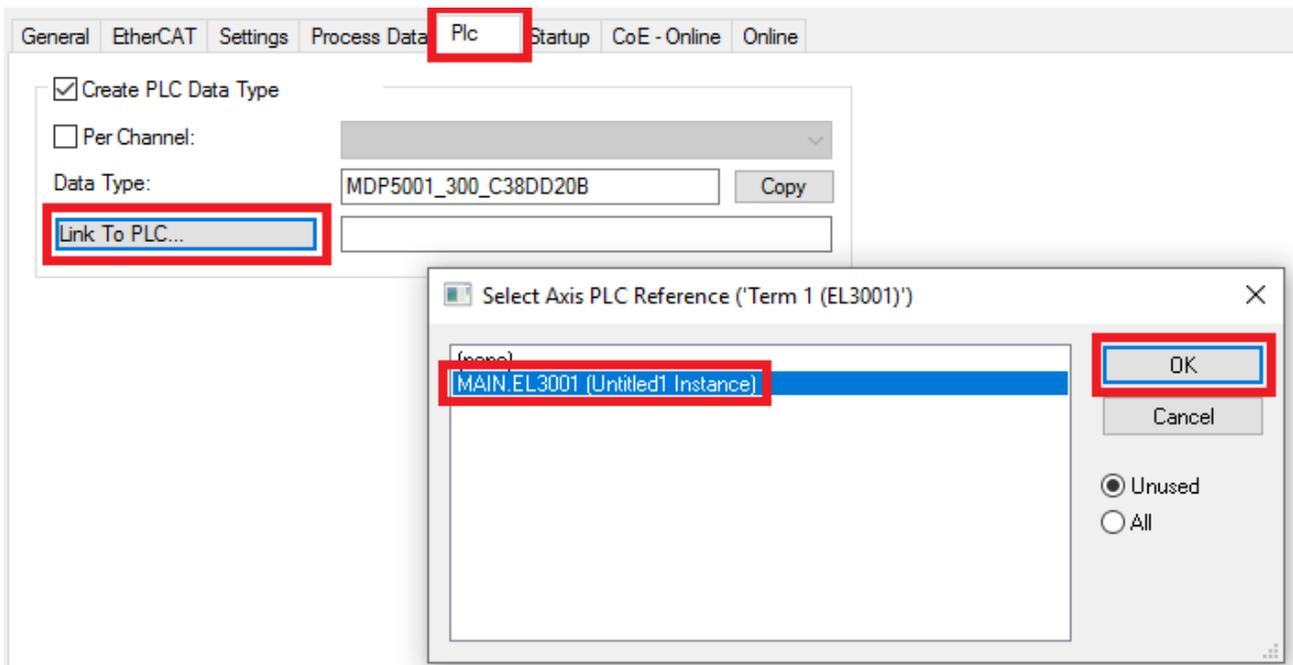
Fig. 63: Linking the structure
