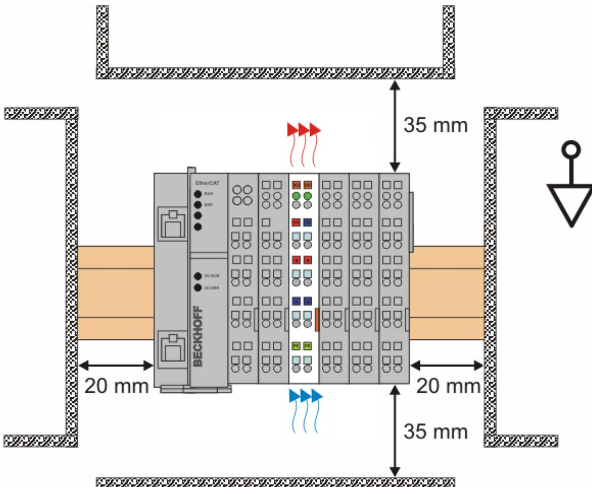
Fig. 20: Recommended minimum distances for standard installation position
