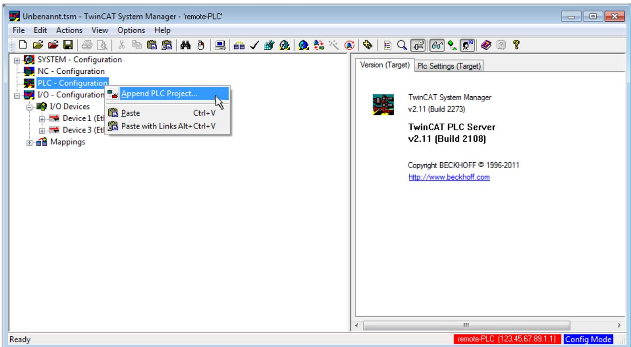
Fig. 35: Appending the TwinCAT PLC Control project
