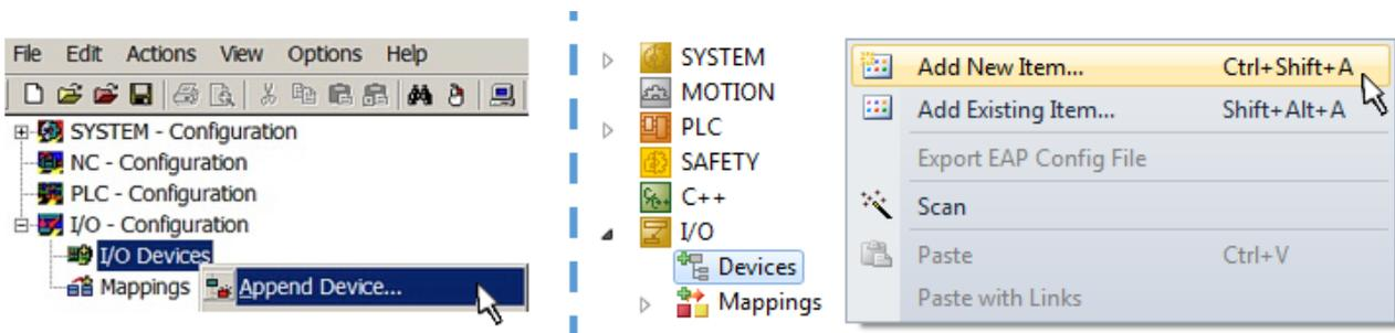
Fig. 83: Append EtherCAT device (left: TwinCAT 2; right: TwinCAT 3)
