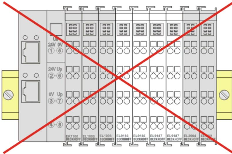
Fig. 22: Incorrect positioning
