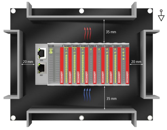
Fig. 15: Recommended distances for standard installation position
