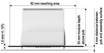
Fig. 14: Mounting distances EJ module - PCB
